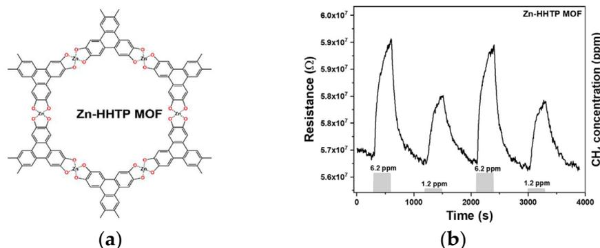
**Figure 1.** (a) Chemical structure of Zn-HHTP MOF; (b) chemiresistive study of Zn-HHTP MOF sensor to 6.2 and 1.2 ppm of CH<sub>4</sub> at room temperature, proving its reversibility.
