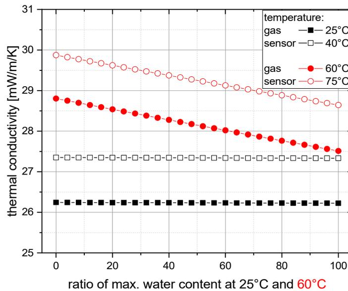
**Figure 2.** Calculated virtual shift in the thermal conductivity when the sensor temperature is 15 K higher than the actual gas temperature. Depending on the starting point in Figure 1, the shift in thermal conductivity is strongly affected by the absolute humidity (60 °C gas temperature).
