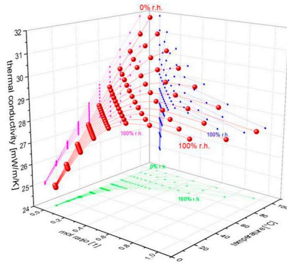
**Figure 1.** Calculated thermal conductivity [3] of humid air as a function of water mol ratio and temperature.
