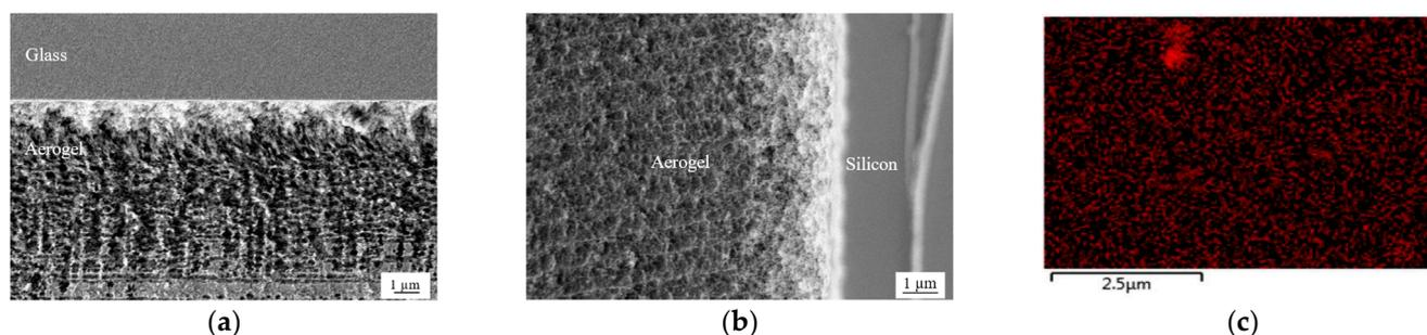
**Figure 1.** View of the chip filled with aerogel, (a) adhesion between glass and aerogel (b) between silicon and aerogel (c) EDX from the middle of the aerogel sample, red dots are Pt nanoparticles.
