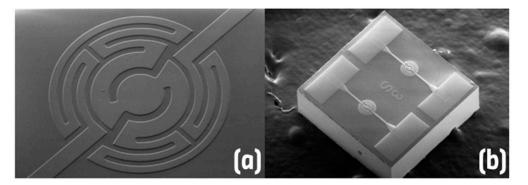
**Figure 1.** Layout of the Pt heater element with a diameter of 150 mm with enhanced temperature homogeneity over the surface (**a**); Microcalorimeter chip with two independent heater elements embedded in separated dielectric membranes (**b**).
