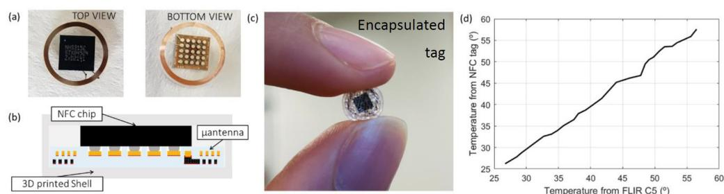
**Figure 2.** (a) Temperature sensing tag before encapsulation, (b) encapsulation schematic, (c) picture of encapsulated tag, and (d) NFC tag temperature measurements against thermal camera readings.
