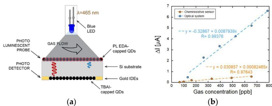
**Figure 1.** (a) Scheme of the optical system architecture; (b) linear fitting of the optical system (blue dots) and chemiresistive sensor (red dots).  $\Delta I = (I_a - I_g)$  for different NB concentrations.
