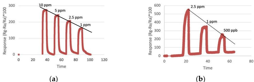
**Figure 1.** Dynamic response curves of sensors  $S_{1\text{Zac-PVA}}$ . (a) Response to NO gas in 1, 2.5, 5, and 10 ppm at 300 °C. (b) Response to NO<sub>2</sub> gas 0.5, 1, and 2.5 ppm at 300 °C.
