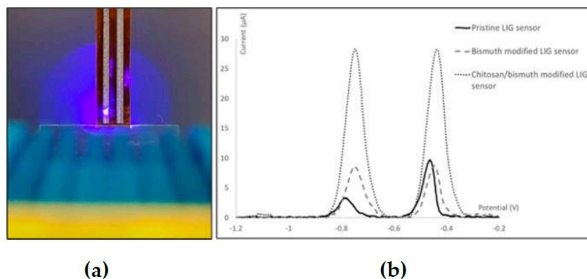
**Figure 1.** (a) Focus on direct patterning of a Kapton tape applied on a PVC substrate: the PI film is converted into a conductive material through the carbonization process operated by a 445 nm laser, in N<sub>2</sub> conditioned atmosphere. (b) Representative responses of pristine, bismuth- and chitosan/bismuth-modified LIG sensors in the simultaneous detection of 25 µg/L of Cd(II) and Pb(II) in KCl solution, pH 2.
