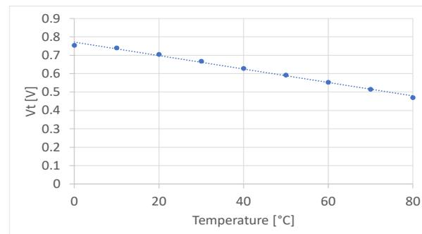
**Figure 2.** Temperature measurement with a MOSFET.
