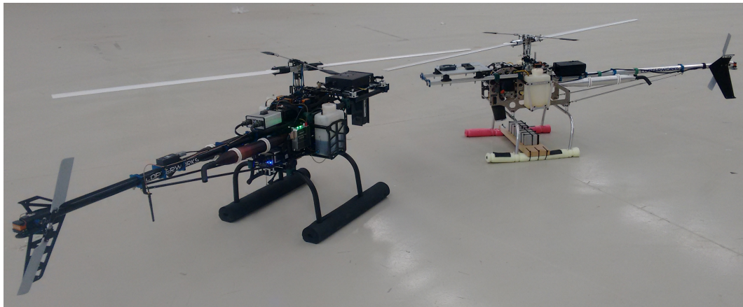
Figure 7. On the left is the fully integrated AF30 and on the right AF25B in radio control mode before the EFI validation test flight. Note the extra weight added on the AF25B model landing gear.
