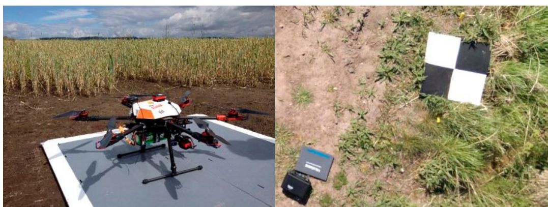
Figure 6. The flexible and cost-effective Tarot 680 Pro hexacopter on a landing pad, with Parrot Sequoia mounted on the underside ( left ); and example of the black and white GCP targets utilised in the field ( right ). © C Moriarty.
