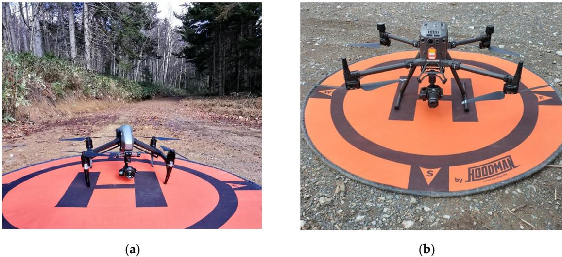
**Figure 2.** (a) DJI-Inspire 2 UAV platform used in Sub-compartment 42B; (b) DJI Matrice 300 RTK UAV platform used in Sub-compartment 16AB.
