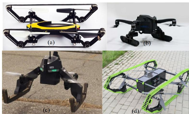
**Figure 39.** Views of tank quadcopter complete with powered treads for terrestrial travel and four rotors for aerial travel, (a) [67], (b) [68], (c) [69], and (d) [70].
