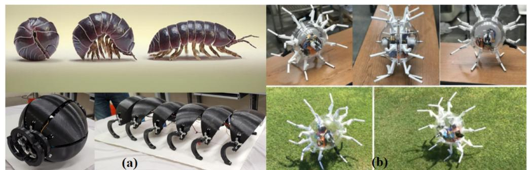
**Figure 21.** View of (a) rolling isopod-based robot demonstrating the conglobation process [34] and (b) golden-wheel-inspired rolling robot [24].
