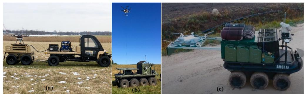
**Figure 46.** Views of tethered drones deployed by military UGVs [92].
