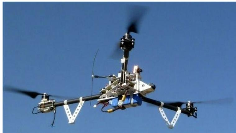
**Figure 30.** Tri-rotor drone in flight [43].
