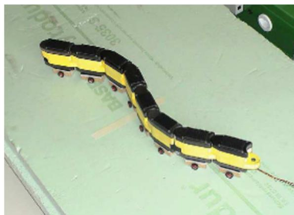
**Figure 14.** Snake-inspired robot with passive wheels controlled by non-linear oscillators which mimic serpentine locomotion [27].
