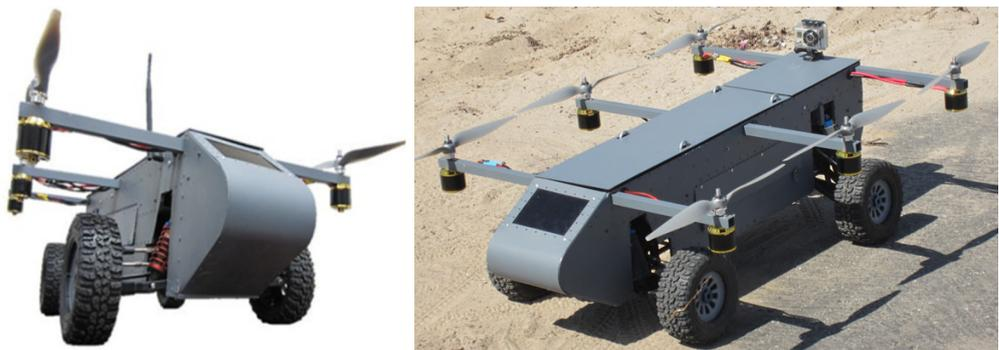
**Figure 43.** Advanced Tactics Panther Drone is one of the first unmanned ground vehicles (UGVs) capable of flight in addition to terrestrial travel. The UGV uses four powered wheels, as well as four rotors that act as a quadcopter with pitch and roll control [76].
