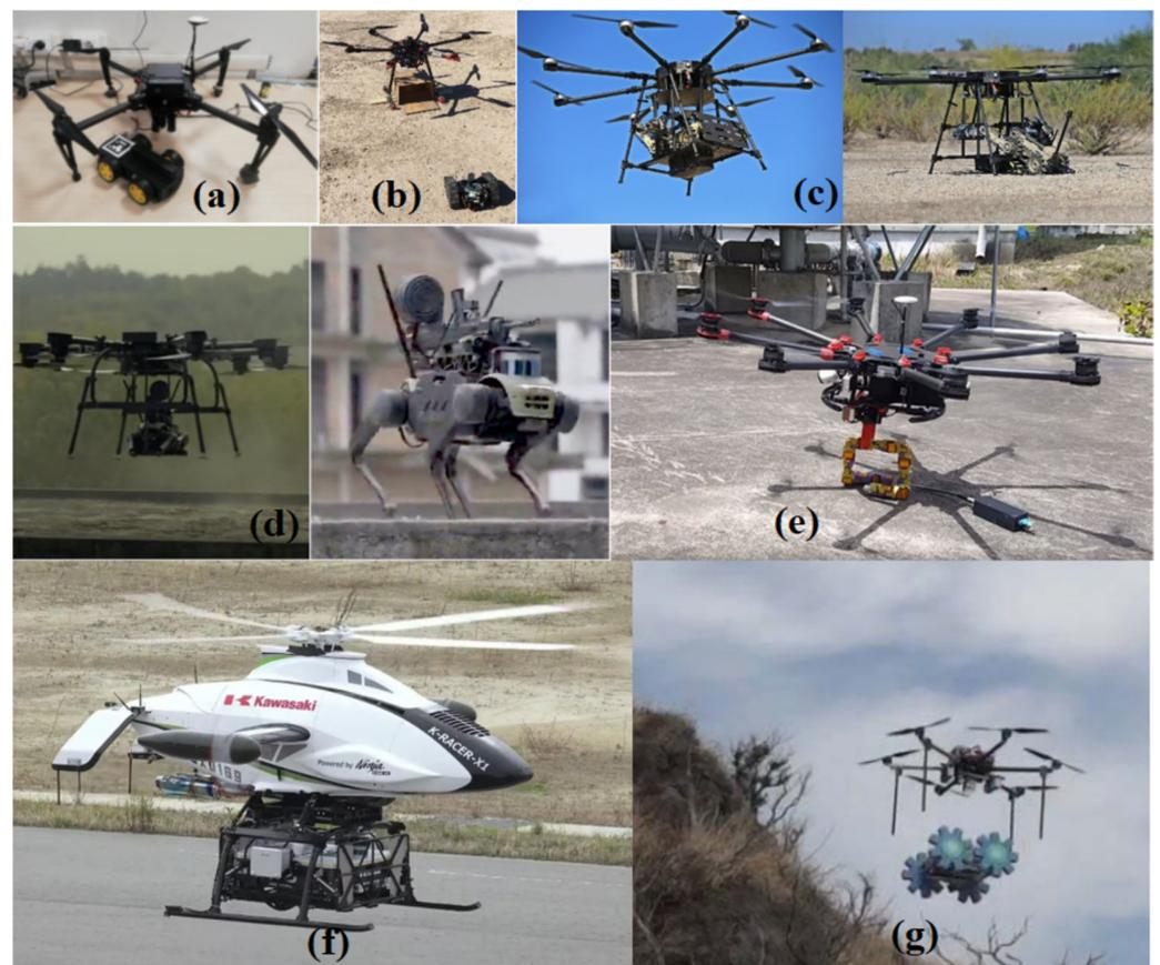
**Figure 53.** View of (a) drone transporting a ground robot [142], (b) team of autonomous drones and UGVs for civil infrastructure inspection [143], (c) a drone that can carry a Micro Tactical Ground Robot (MTGR) [144], (d) drone deploying a quadrupedal unmanned ground vehicle [145], (e) a drone that can carry a snake robot for accident monitoring [146], (f) autonomous helicopter which transport a cargo robot [147], and (g) a robotic systems for volcano exploration [148].
