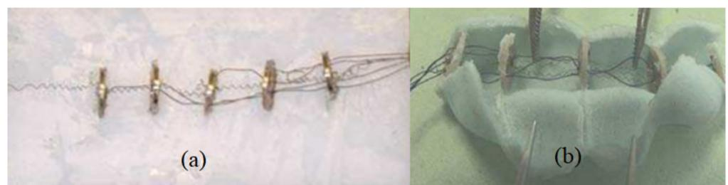
**Figure 16.** View of (a) shape-memory alloy skeleton of robotic earthworm design and (b) wrapped in a Nylon mold [29].
