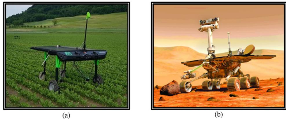
**Figure 2.** Examples of wheeled UGVs with specialized functionalities: (a) four-wheeled UGV drives through seedlings, picking weeds between rows [13]; (b) six-wheeled UGV traverses Mars' surface.
