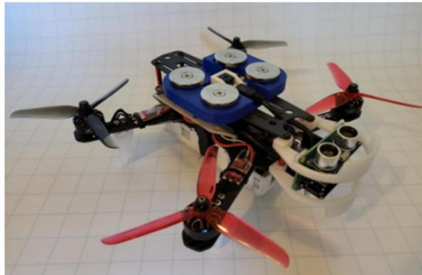
**Figure 32.** Semi-autonomous precision-docking quadcopter constructed from a racing drone frame with custom sensors and flight controllers [45].
