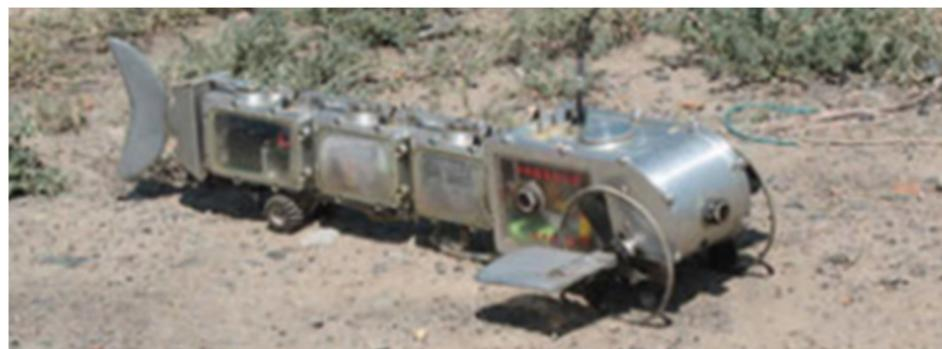
**Figure 23.** Mechanism design of AmphiRobot-II; prototype of the amphibious robot in the field test [36].
