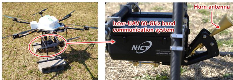
Figure 3. Photographs of the UAV and onboard equipment utilized in this demonstration.
