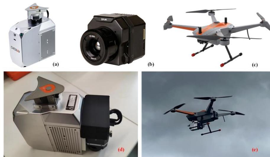
**Figure 1.** Establishing multi-sensor equipment on UAV platform. (a,d) AlphaAir 450 pocket LiDAR system; (b) FLIR VUE Pro R camera; (c) BB4 mini UAV; (e) multi-sensor equipment on UAV platform.
