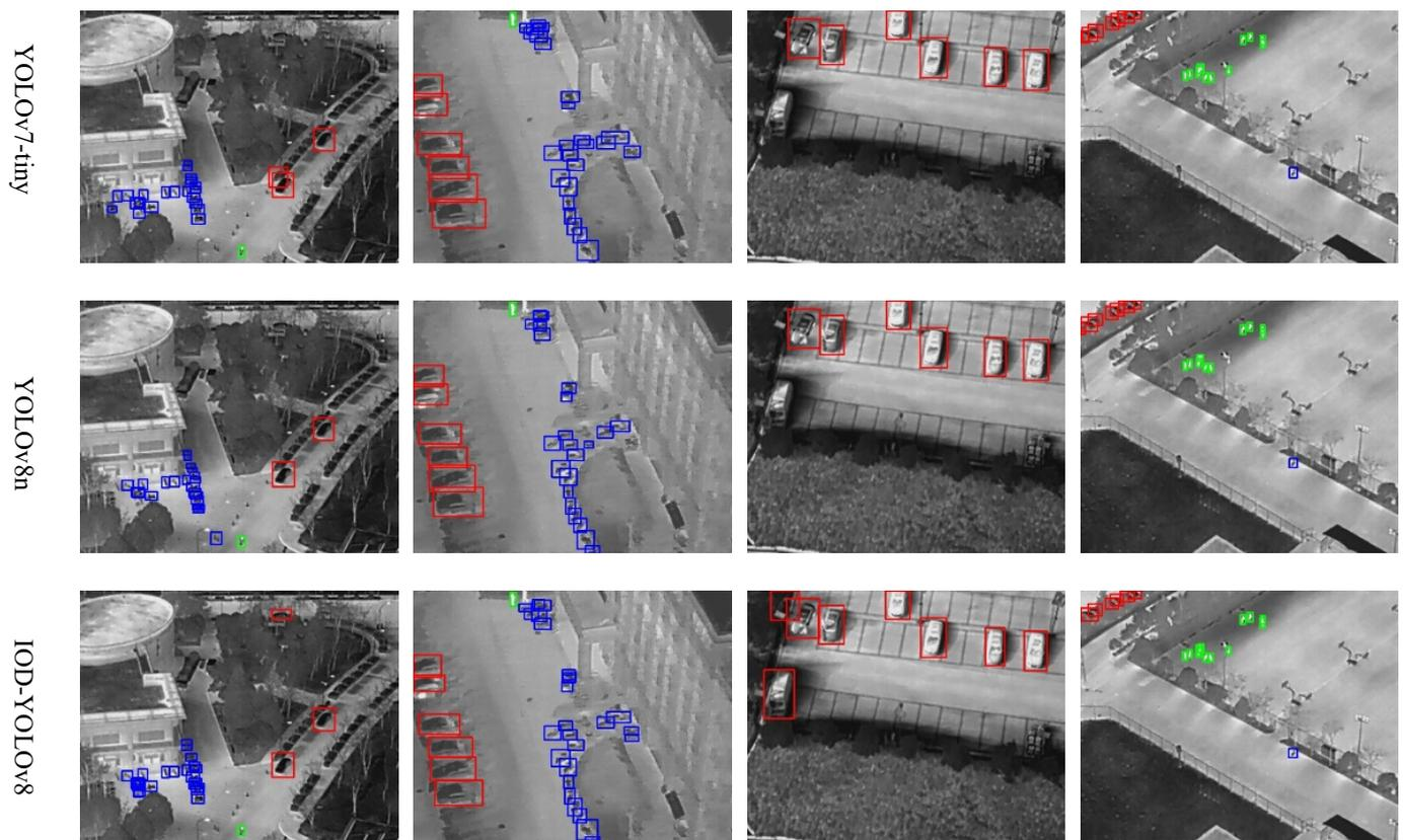
**Figure 7.** Comparison of the visualization results of different algorithms, where the vehicle target is represented by a red box, and the bicycle and person targets are represented by blue and green boxes, respectively.
