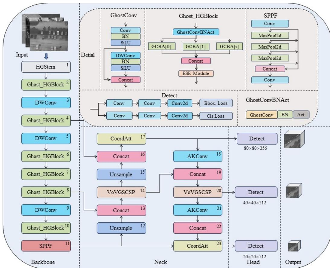
Figure 1. ITD-YOLOv8 network structure diagram.
