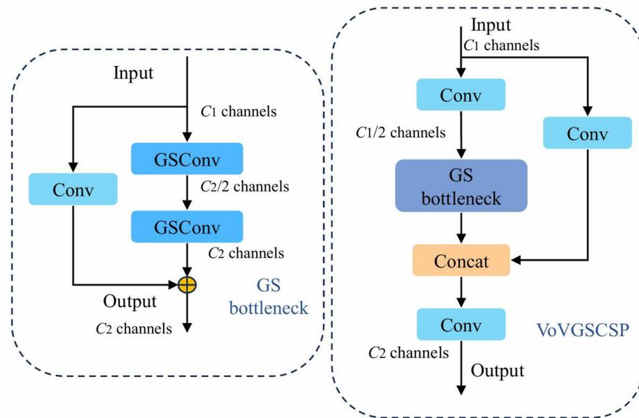
Figure 3. Structure of the VoVGSCSP module.
