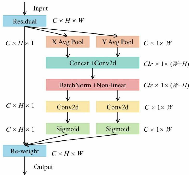
Figure 5. Structure of the attention mechanism CoordAtt.
