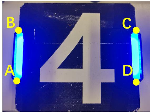
**Figure 2.** Armor (light bars are the main visual features; A, B, C, and D are four points used for solving pose).
