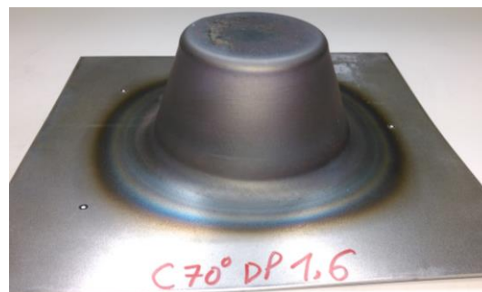
Figure 10. A 70^\circ cone wall angle by a varied feed rate made form HCT980C steel.
