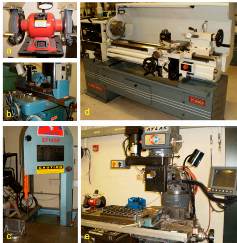
Figure 1. Test machines for acoustic emission: (a) bench grinder; (b) surface grinder; (c) vertical band saw; (d) lathe machine; and, (e) vertical milling machine.
