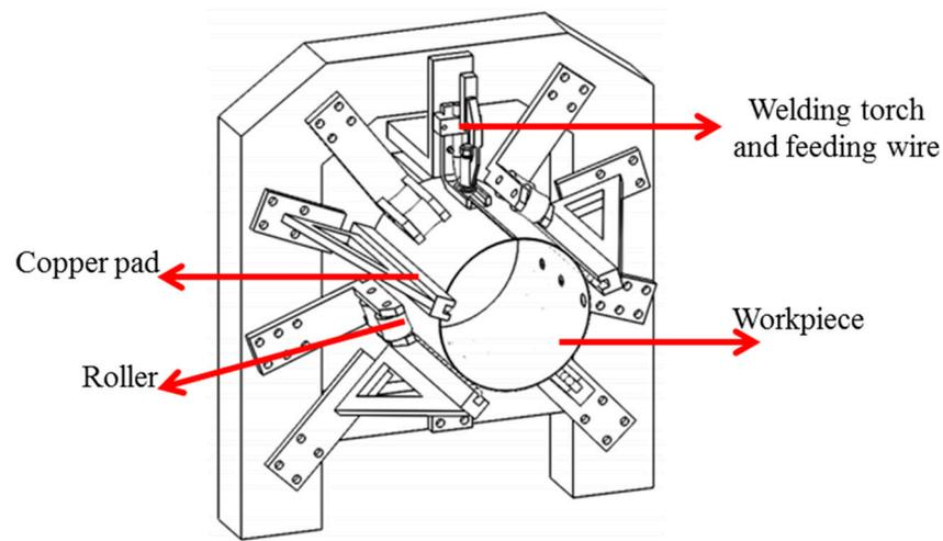
**Figure 1.** Plasma welding system isometric drawing.
