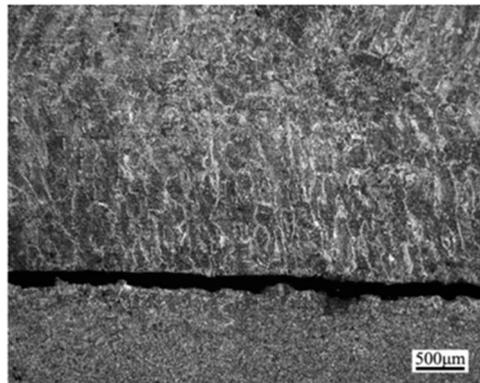
**Figure 8.** Crack morphology of longitudinal weld after pressure pulse test.
