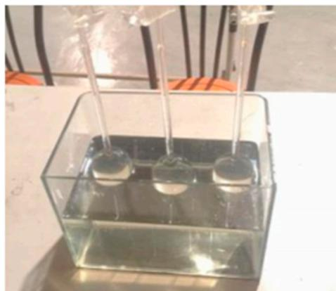
**Figure 6.** Device for diffusible hydrogen testing.
