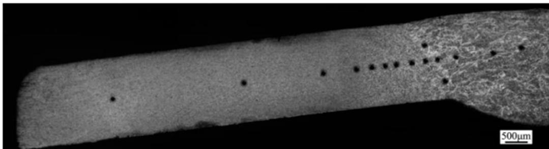
**Figure 10.** Points selection for micro-hardness test of longitudinal weld.
