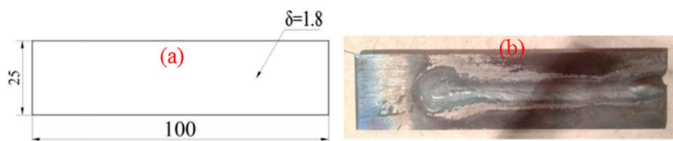
**Figure 5.** Diagram of test block (a) and surface of welded block (b) used for the diffusible hydrogen testing.
