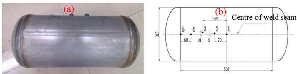
**Figure 3.** Physical picture (a) and measurement sites for the tank (b) under test.
