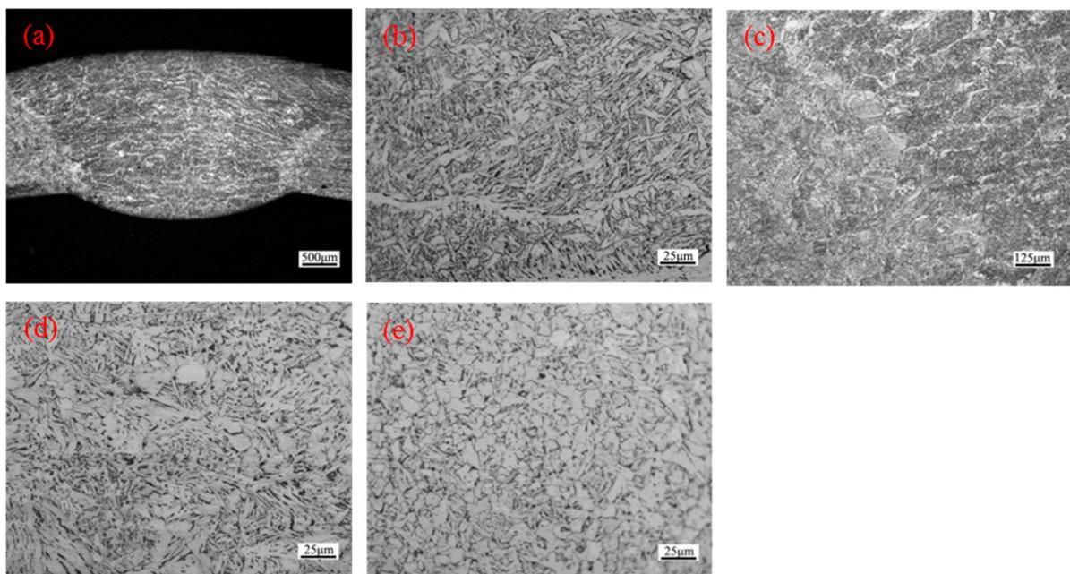
**Figure 7.** Micro-structure of electric water heater tank longitudinal weld: (a) weld zone (b) Columnar grain zone in the middle of weld (c) Fusion zone (d) Heat affected zone (superheated zone) (e) Heat affected zone (normalized zone).
