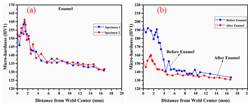
**Figure 15.** Micro-hardness distribution of longitudinal weld (a) after enameling (b) contrast of before and after enameling.
