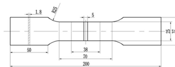
**Figure 2.** Specimen for tensile strength test of longitudinal weld.
