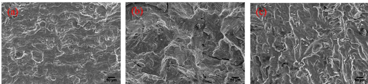
**Figure 9.** SEM morphology of longitudinal weld fusion line crack (a) initial crack zone; (b) propagation zone and (c) final fracture zone.
