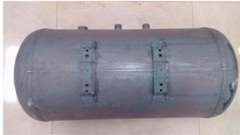
**Figure 13.** Electric water heater tank after enameling.
