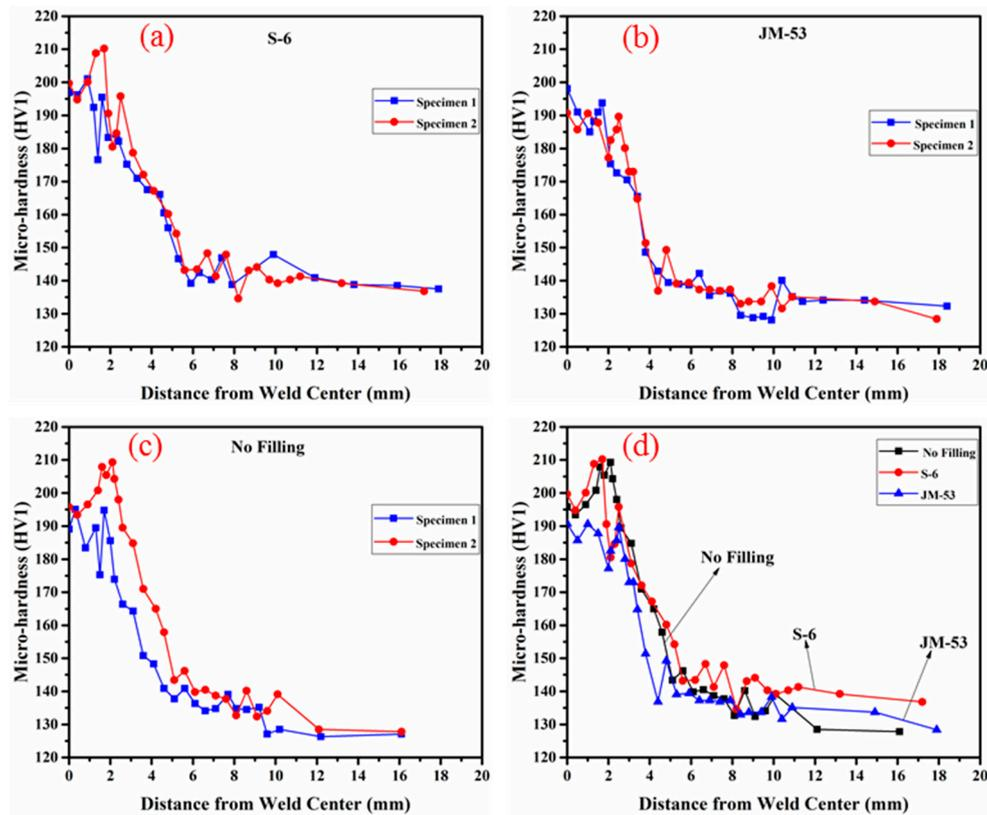
**Figure 11.** Micro-hardness distribution of welds using different welding wires (a) S-6; (b) JM-53; (c) No Filling; and (d) All.
