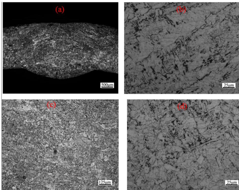
**Figure 14.** Microstructure of longitudinal weld after enameling (a) weld zone; (b) weld columnar grain; (c) fusion zone; and (d) heat affected zone.
