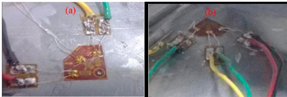
**Figure 4.** Connection modes of strain gauge lead in longitudinal and transverse directions (a) and removal of strain gauge lead (b).
