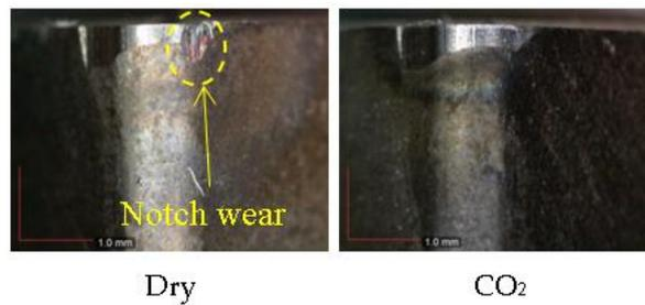
**Figure 6.** Images of notch wear occurring after 500 mm cutting length.
