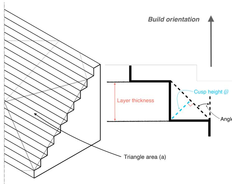
**Figure 7.** Cusp height, generated by difference between the nominal and real model, as simple and analytic evaluation of surface quality.
