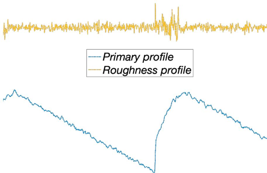
**Figure 8.** Qualitative plots describing the primary profile and roughness profiles, as defined by ISO 4287 [60], of the real profile of an AM component characterized by a significant stair-stepping effect.
