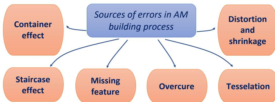
Figure 3. Sources of errors in Additive Manufacturing (AM) building process described in [23].
