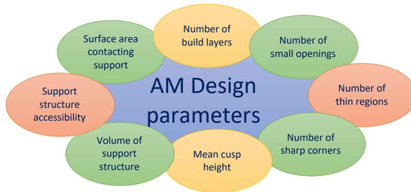
**Figure 6.** Design parameters considered in the optimization model for build orientation used in [22].
