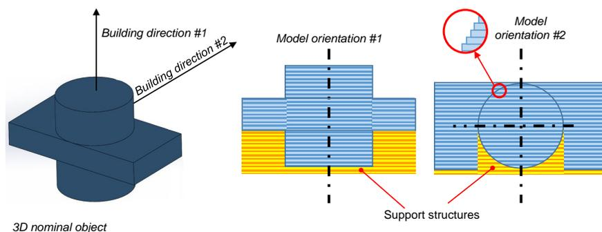
**Figure 2.** Stair-stepping effect and supports structure: effect of the build direction.
