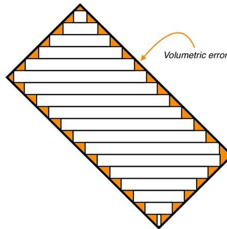
Figure 4. Graphical visualization of volumetric error.
