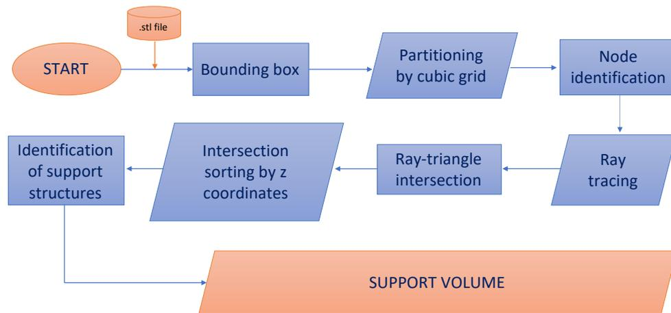
Figure 9. Flowchart of the voxelization algorithm proposed by [40].
