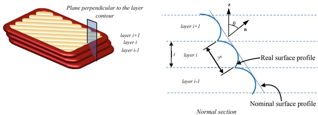
**Figure 1.** Stair-stepping effect: the nominal surface and the real surface are not coincident.
