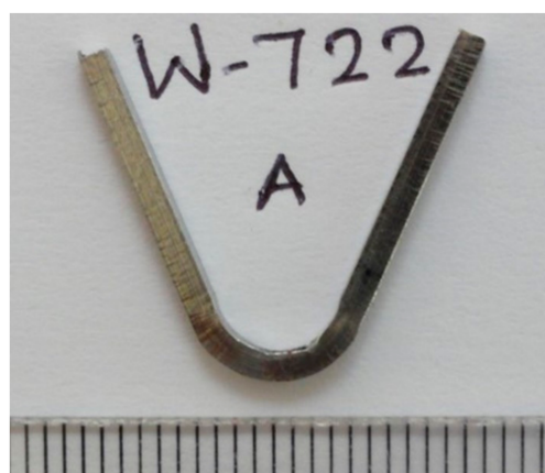
Figure 12. Typical face bent specimen.
