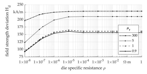
**Figure 13.** Field strength deviation  $H_d$  (standard deviation of the magnetic field strength) in the workpiece in respect of the specific resistance of the die material.
