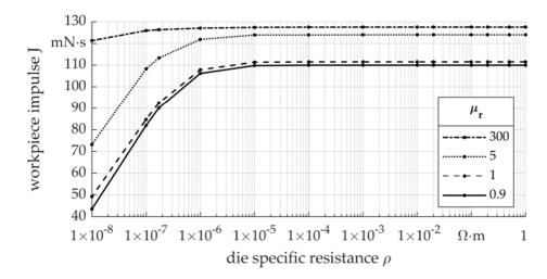
**Figure 6.** Simulated impulse *J* on thin aluminium sheets for different electromagnetic properties of the die material.
