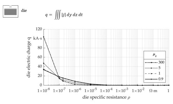
**Figure 8.** Integral of the current density j in the die volume over time in respect of the specific resistance  $\rho$  of the die material.
