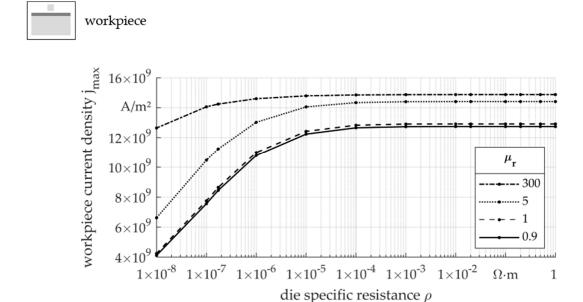
**Figure 7.** Maximum current density  $j_{max}$  in the workpiece volume in respect of the specific resistance  $\rho$  of the die material.
