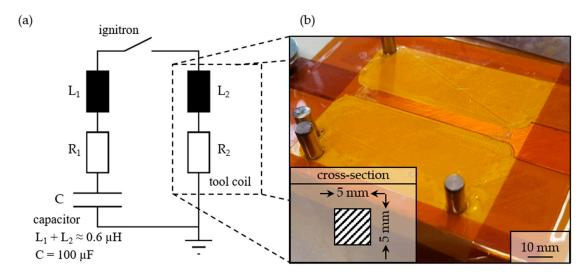
Figure 2. Experimental setup; (a) equivalent circuit diagram; (b) tool coil.
