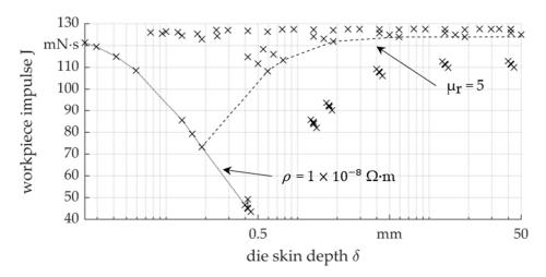
**Figure 5.** Simulated impulse as a function of the resulting skin depth for the parameter combination of specific resistance  $\rho$  and relative permeability  $\mu_r$  values.
