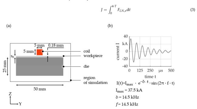
Figure 1. Simulation model; (a) schematic; (b) input current (tool coil).
