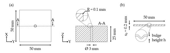
Figure 3. Forming experiment; (a) free forming die geometry; (b) resulting workpiece geometry.
