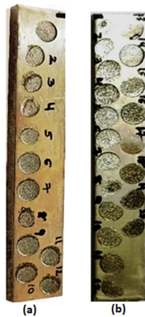
Figure 4. Sample work pieces after machining. (a) Ti-6Al-4V. (b) SS316.
