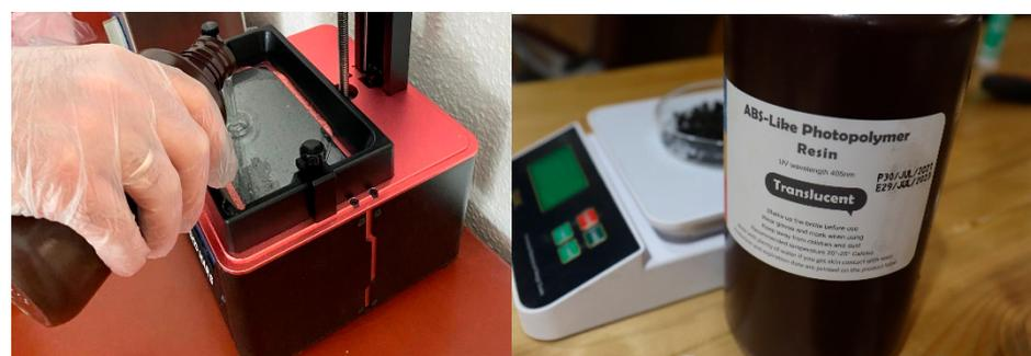
**Figure 2.** ABS-like photopolymer resin used in the study.
