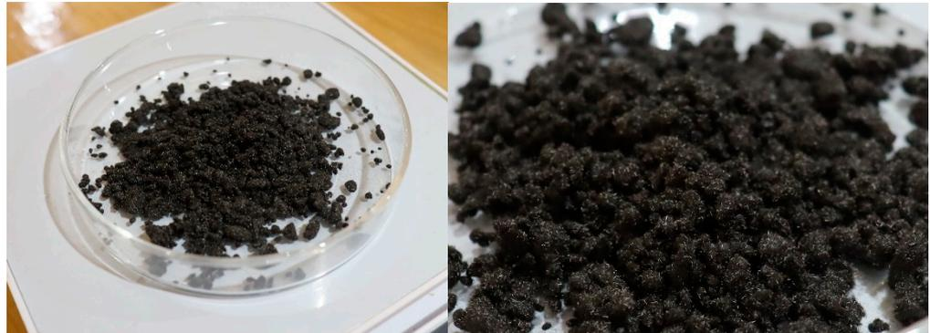
**Figure 1.** Milled carbon fiber,  $100 \mu\text{m}$ .
