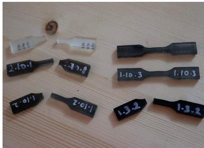
Figure 10. Dog-bone tensile specimens before and after tensile test.
