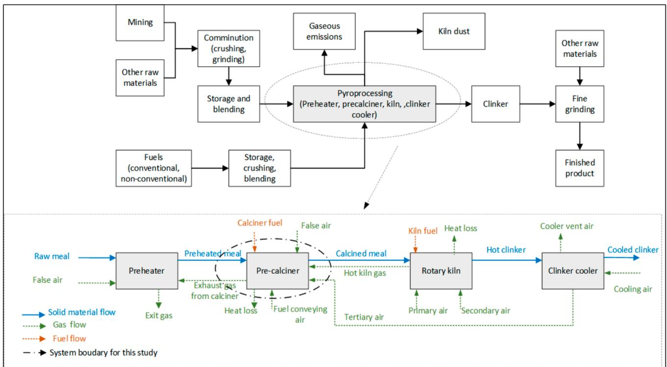
**Figure 3.** Flow stream input/output information is shown in a schematic representation of a typical cement production facility for the pyro-processing phase [23].
