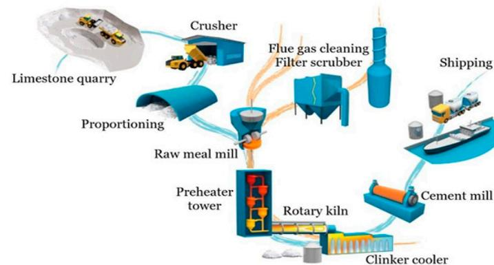
**Figure 1.** Diagram of the general procedure at the cement plant. Adapted from P. del Strother [11].
