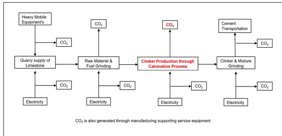
**Figure 4.** Simple cement manufacturing processes showing the CO<sub>2</sub> generation systems.
