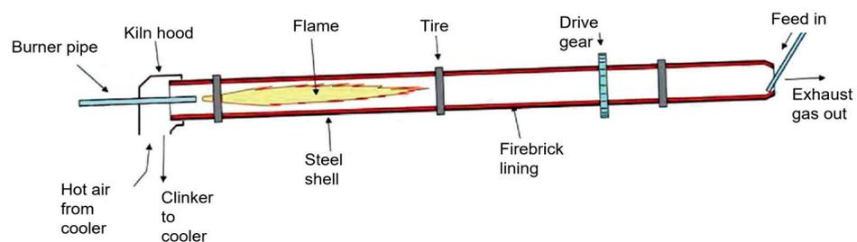
**Figure 2.** The rotary kiln’s general design [18].
