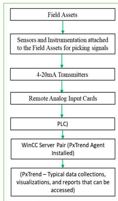
**Figure 8.** Typical instrumentation data system and data collection setup for Heidelberg Material Union Bridge Cement Plant [10,61].
