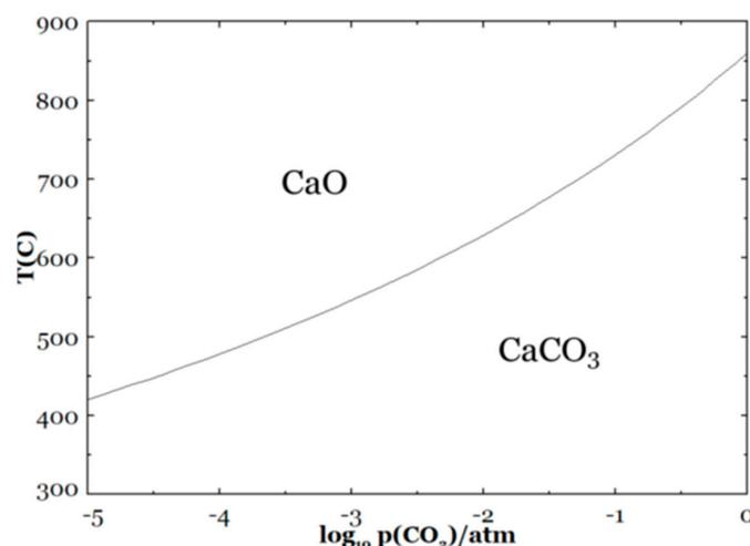
**Figure 5.** Calcium carbonate calcination temperature as a function of carbon dioxide partial pressures at 1 atm. Calculated with FactSage 8.0 software [30,36].
