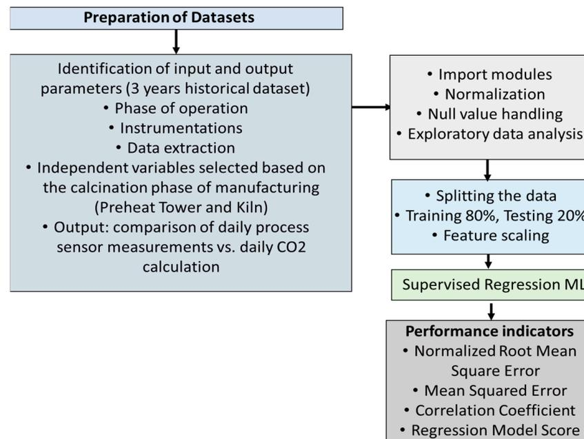
Figure 9. The workflow used for the ML.
