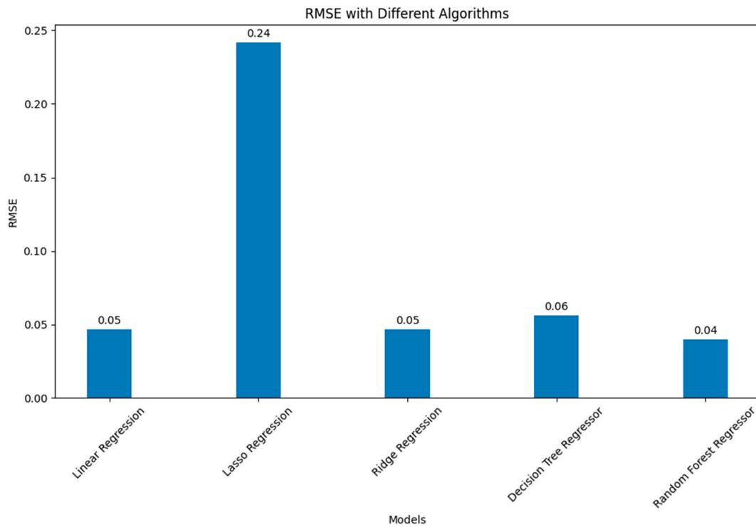
Figure 18. The normalized RMSE with different algorithms for the predictive modeling.
