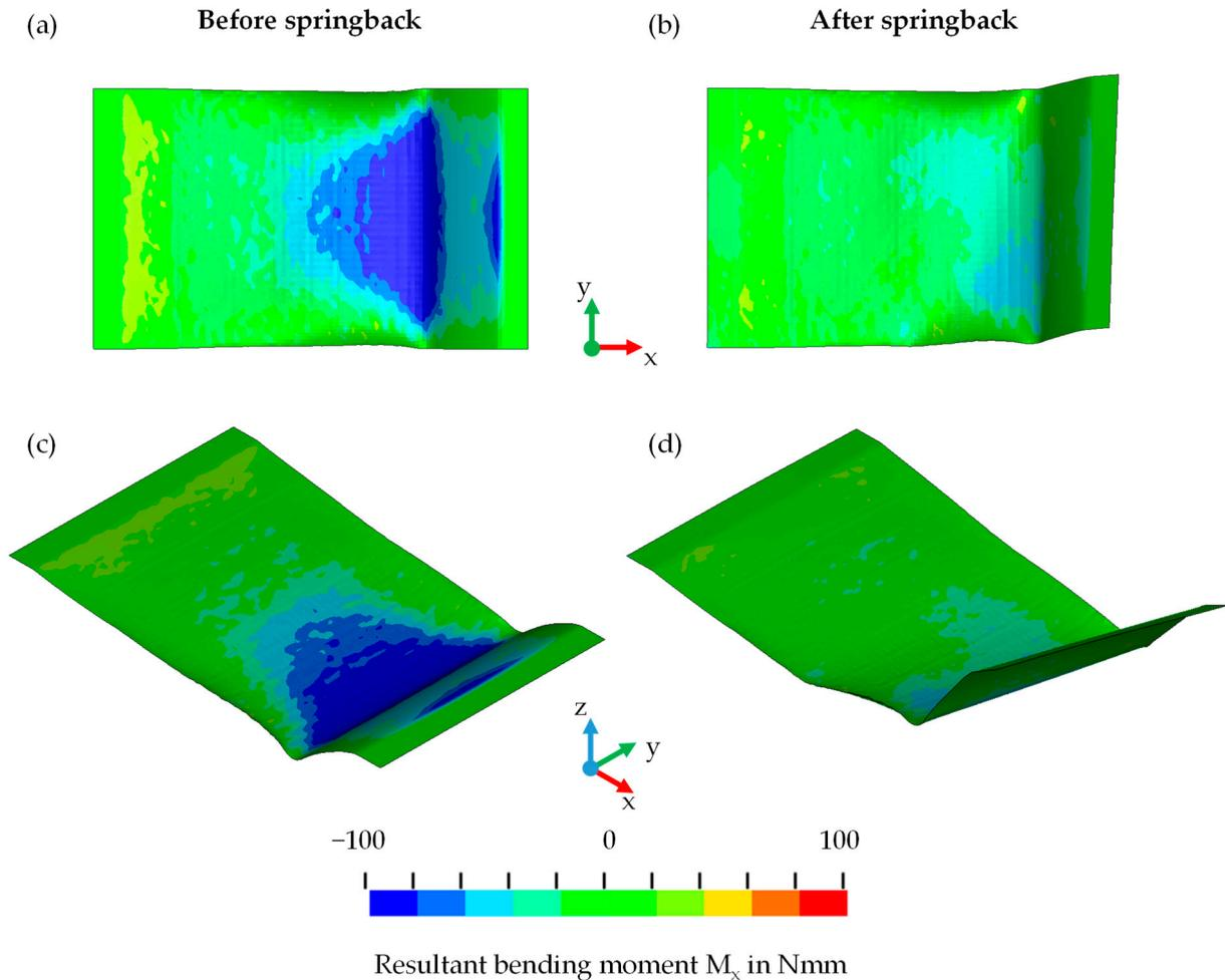
**Figure 12.** Resulting bending moments  $M_x$  for an exemplary linear tool path in top-view (a,b) and ISO view (c,d), before springback (a,c), and after springback (b,d).
