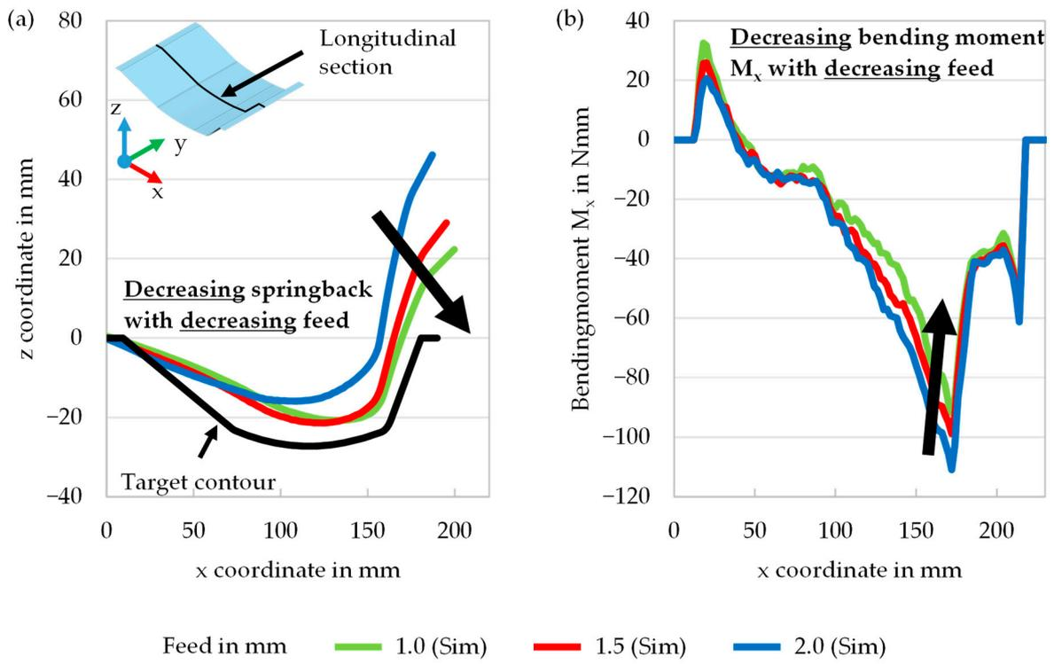
Figure 14. (a) Influence of the feed on the springback and (b) the resulting bending moment  $M_x$  before springback.
