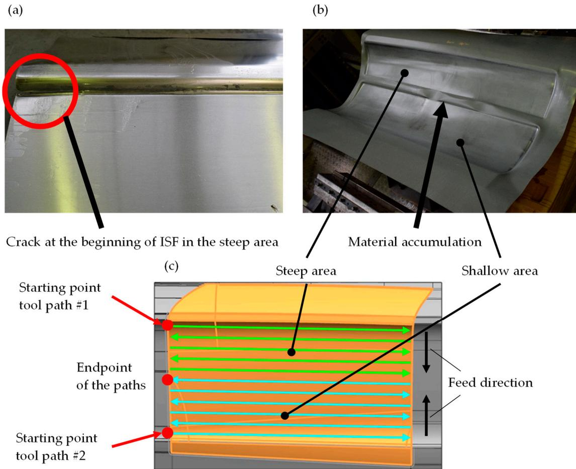
**Figure 4.** (a) Crack at steep wall angle using AlMg3. (b) After unclamping: no crack, but material accumulation in the middle area of the component using a mild steel. (c) Schematic representation of a streamlined path strategy (top view).
