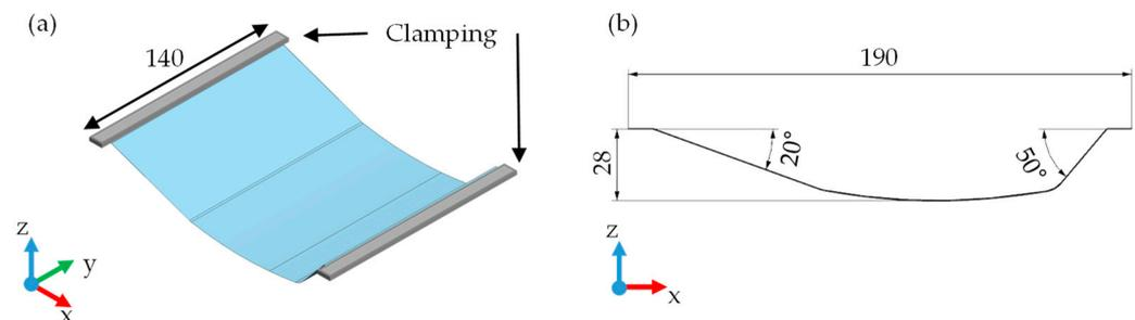
**Figure 3.** Schematic overview of the designed benchmark geometry: (a) ISO-view, (b) longitudinal section (units in mm).
