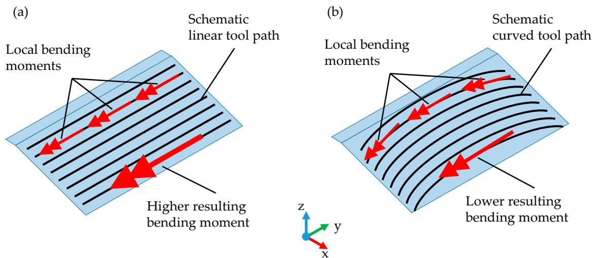
**Figure 2.** Schematic illustration of a hypothesis on resulting residual bending moment along (a) linear tool path and (b) curved tool path.
