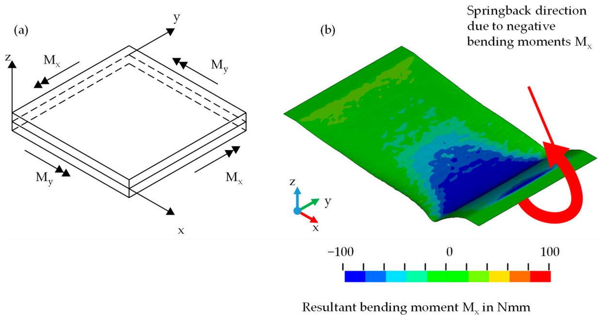
**Figure 11.** (a) Sign convention of the bending moments  $M_x$  and  $M_y$  and (b) exemplary representation of the resulting bending moment  $M_x$  after forming.
