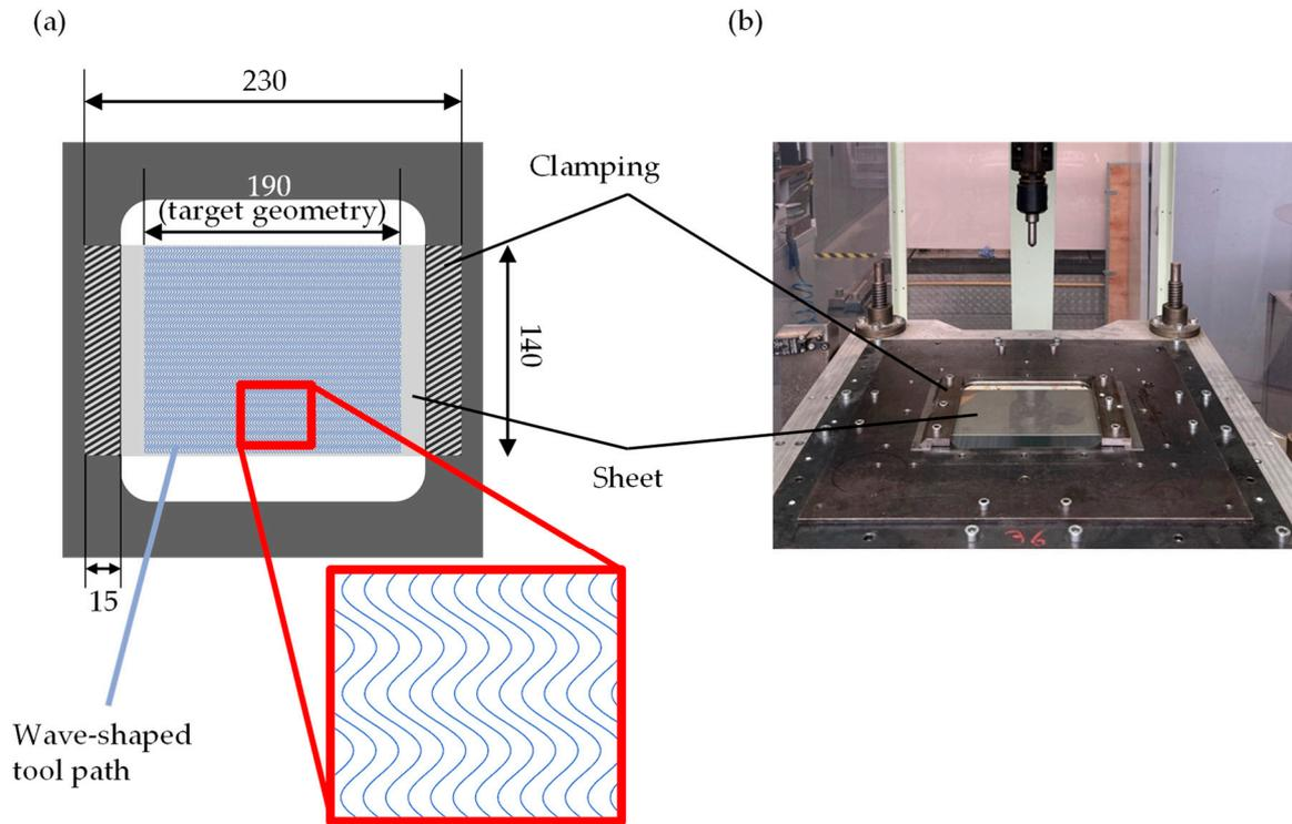
**Figure 6.** (a) Schematic experimental setup: wave-shaped tool path (blue lines, magnified view in red box), (b) experimental setup with clamped sheet (units in mm).
