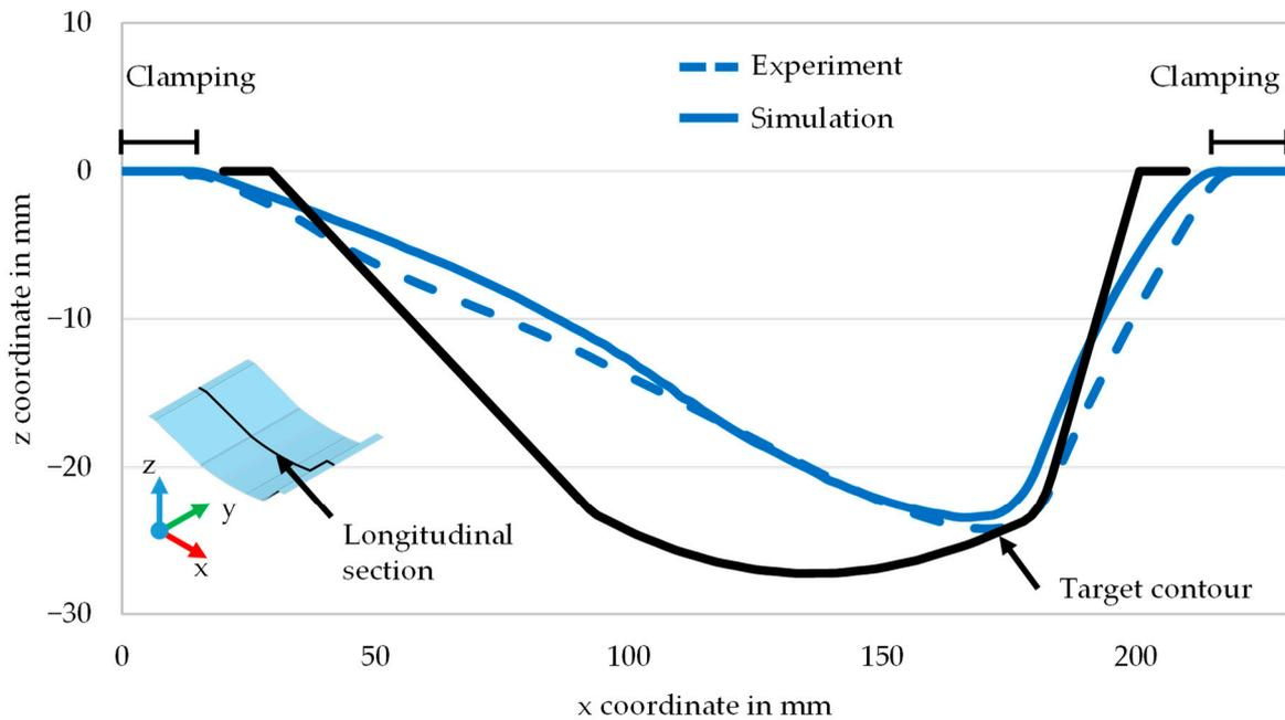
**Figure 7.** Comparison of results after forming between experimental and numerical results with linear tool paths (tool diameter 20 mm; feed 2 mm).
