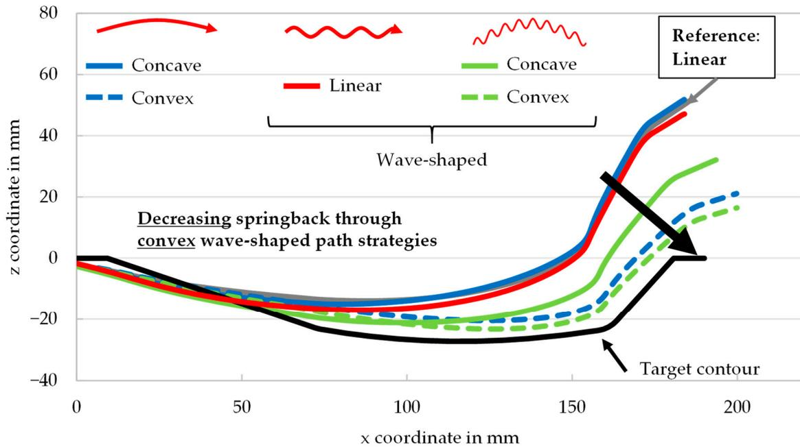
Figure 9. Experimental results on the influence of selected wave-shaped tool path strategies on the springback compared to a linear tool path (feed: 1.5 mm).
