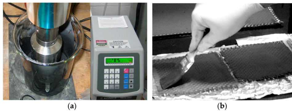
Figure 1. (a) Preparation of graphene solution through ultrasonication; (b) graphene coating process onto plain weave glass fabric.
