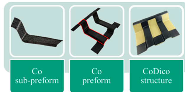
Figure 1. Example of a local continuous fiber reinforced composites (CoFRP, black) reinforced discontinuous fiber reinforced composites (DiCoFRP, white) structure (obtained from [1]).
