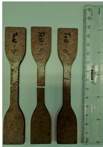
Figure 4. Tensile tested samples cut from WPC panel in 0°, 45° and 90°.
