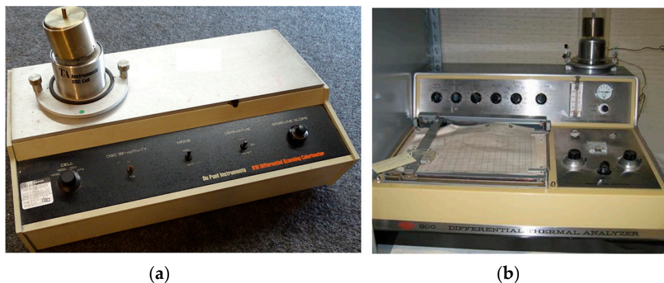
Figure 6. Differential thermal analyzer (a) and differential scanning calorimetry (DSC) analyzer (b) for the measurement of interphase thickness.
