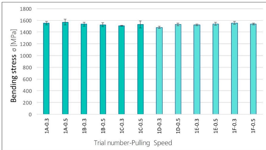
Figure 5. Bending stress for different pulling speeds and resin mixing times.
