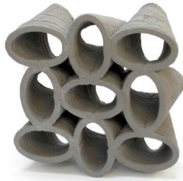
**Figure 9.** 3D printed acoustic damping wall (Reproduced with permission from: [44], Materials and Design; published by Science Direct, 2016).
