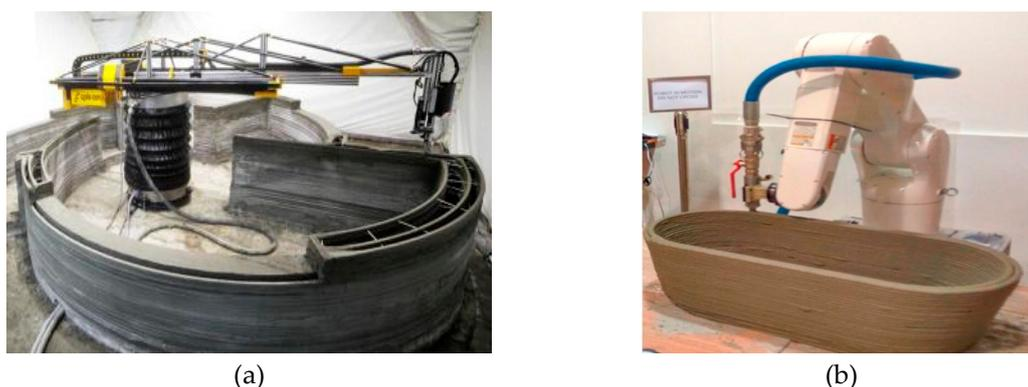
**Figure 3.** (a) Apis Cor 3D printer (Reproduced from [12]) and (b) SC3DP six-axis robot (Reproduced with permission from: [16], Virtual and Physical Prototyping; published by Taylor & Francis Group, 2017).
