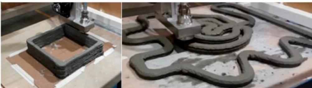
**Figure 7.** Additive Manufacturing as Walls 3D Manufacturing and Bricks 3D Manufacturing. (Reproduced with permission from: [16], *Virtual and Physical Prototyping*; published by Taylor & Francis Group, 2017).
