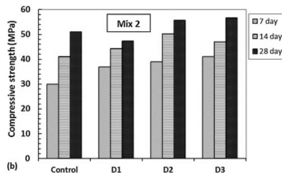
**Figure 6.** Compressive strength of 3D printed samples at different direction loading. (Reproduced with permission from: [7], Archives of Civil and Mechanical Engineering; published by Science Direct, 2018).
