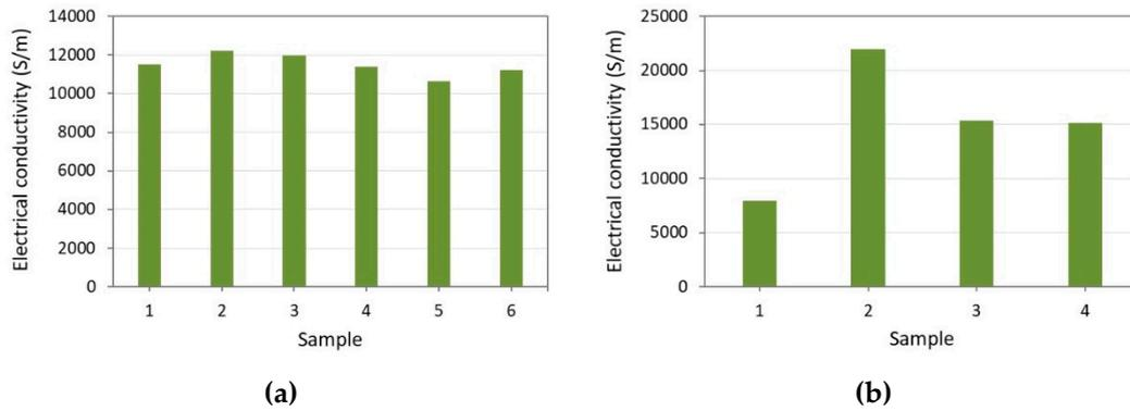
Figure 6. Electrical conductivity values of bio-composites: (a) CF-Rosin; (b) CF-Flax/Epoxy.
