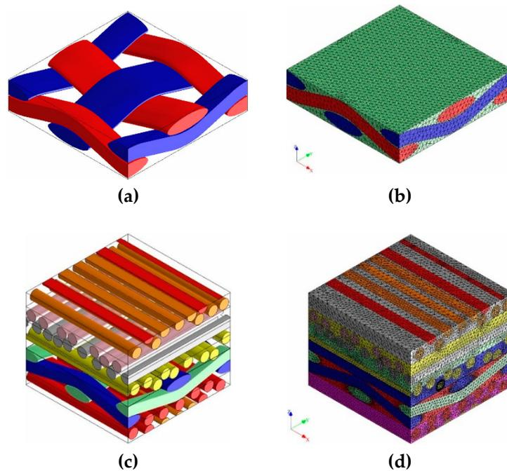
**Figure 5.** (a) RVE of CF/Rosin bio-composite (twill carbon fabric); (b) FE mesh of the RVE of CF/Rosin bio-composite; (c) RVE of CF/Flax-Resin bio-composite; (d) FE mesh of the RVE of CF/Flax-Resin bio-composite.
