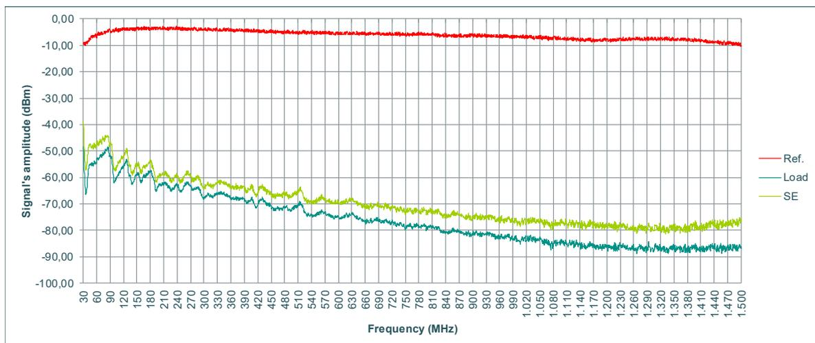
Figure 8. Signal's amplitude vs. frequency for the CF/Rosin bio-composite.
