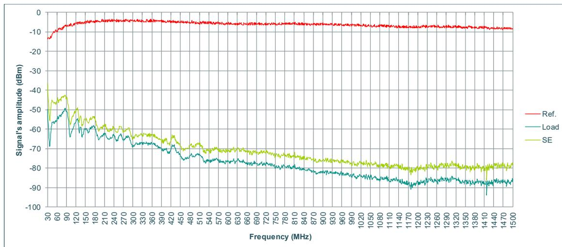
Figure 9. Signal's amplitude vs. frequency for the CF/Flax-Epoxy bio-composite.
