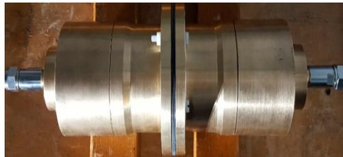
**Figure 4.** The specimen apparatus used for the EMSE tests.
