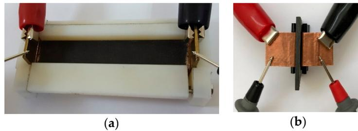
**Figure 1.** (a) The electrical resistivity test along the X axis; (b) the electrical resistivity test along the Z axis.
