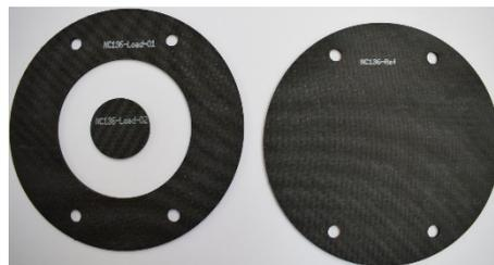
**Figure 2.** The specimens used in the EMC (electromagnetic compatibility) tests (left: reference; right: load).
