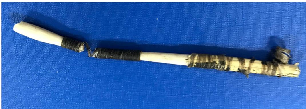
**Figure 6.** Failure occurs within the link-shaft joint under impact, while the bone arrowhead, the bone balance and the main shaft remain intact.
