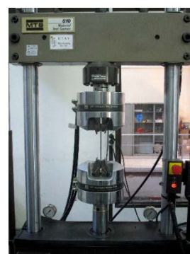
Figure 4. (a) Geometry and dimensions of the scarfed sample; (b) photograph showing a scarfed specimen under tensile loading.
