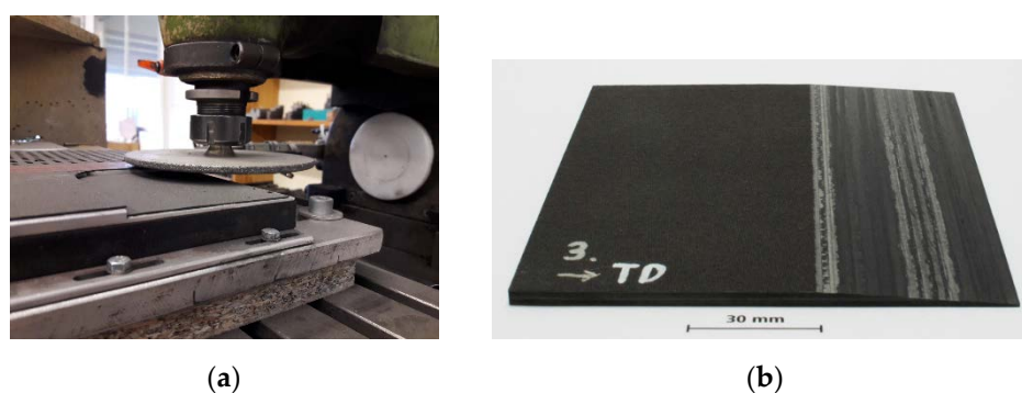
Figure 2. (a) Milling device; (b) overview of scarfed sample after milling.
