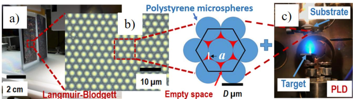
**Figure 1.**  $\text{VO}_2$ -Ir microtriangles composites' manufacturing pathway. (a) Photography of a perpendicular substrate covering by polystyrene spheres (P-spheres). (b) Schematic of spheres (P-spheres) compact arrangement. (c) Photography of a pulsed laser deposition process.
