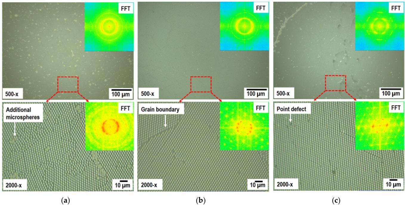
**Figure 2.** Temperature dependence of the 2D arrangement of polystyrene microspheres (P-spheres) with a 3-micrometer diameter on an  $\text{Al}_2\text{O}_3\text{-c}$  substrate: (a) P-spheres deposited at 20 °C using Langmuir–Blodgett colloidal lithography (LB); (b) P-spheres deposited at 25 °C using LB; (c) P-spheres deposited at 30 °C using LB. The insert images in Figure 2 represent the Fast Fourier transform (FFT) of the underlying optical images of the LB results.
