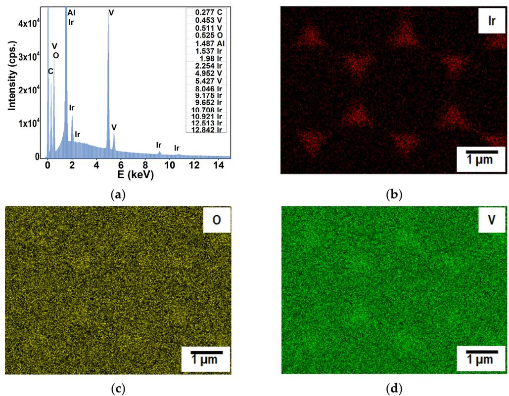
**Figure 4.** Energy Dispersive X-ray Spectroscopy and Elemental mapping of a VO<sub>2</sub>–Ir composite. The thickness of VO<sub>2</sub> 200 nm and the “a” parameter of Ir microtriangles is equal to 0.70 μm (a) EDS elemental analyses of the composite; (b) Elemental map of Ir microtriangles; (c) Elemental map of Oxygen; (d) Elemental map of Vanadium.
