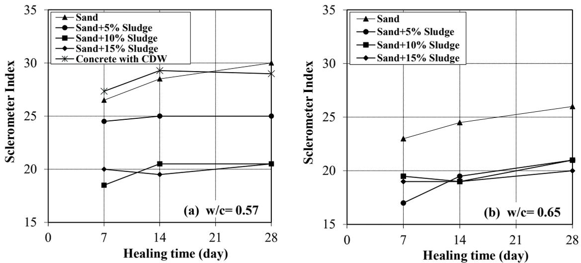
**Figure 7.** Sclerometer index versus healing time: (a) conventional concrete, with sewage sludge and with CDW [27],  $w/c = 0.57$  and (b) conventional concrete with sewage sludge,  $w/c = 0.65$ .
