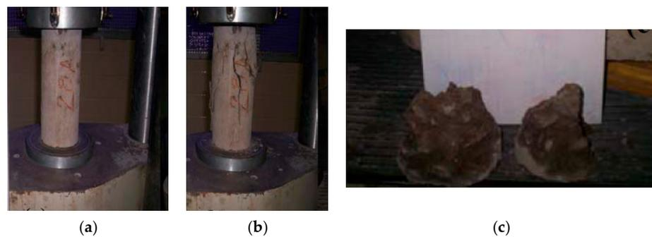
**Figure 2.** Compressive strength test view: (a) sample in the press, (b) broken sample, and (c) rupture of the specimen (age of 28 days and 15% sludge).
