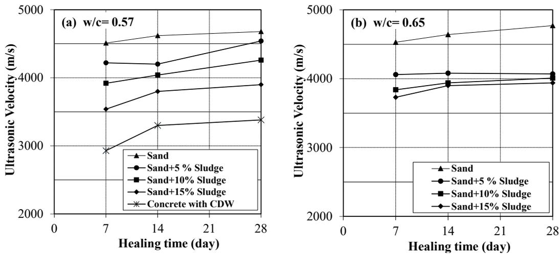
**Figure 6.** Ultrasonic velocity versus healing time for: (a) conventional concrete, concrete with sewage sludge, and with CDW [27] for  $w/c = 0.57$ ; and for (b) conventional concrete and concrete with sewage sludge for  $w/c = 0.65$ .
