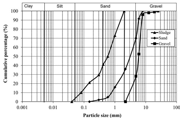
**Figure 5.** Particle size distribution of the aggregates.
