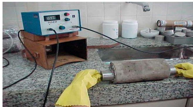
**Figure 3.** Ultrasonic Velocity Test.
