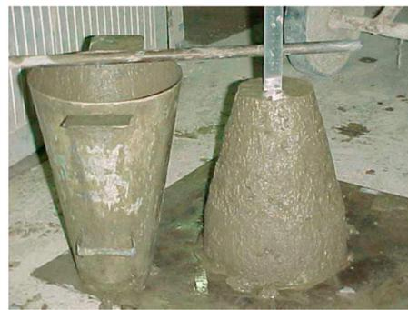
**Figure 1.** Slump cone test method.
