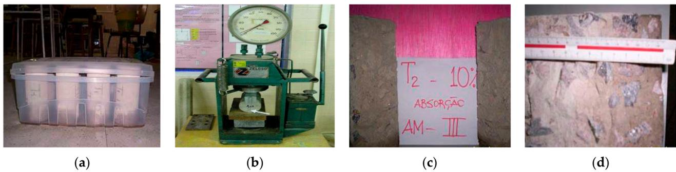
**Figure 4.** Capillary absorption test: (a) specimen immersed in water; (b) hand press; (c) broken specimen; (d) absorption by the specimen.
