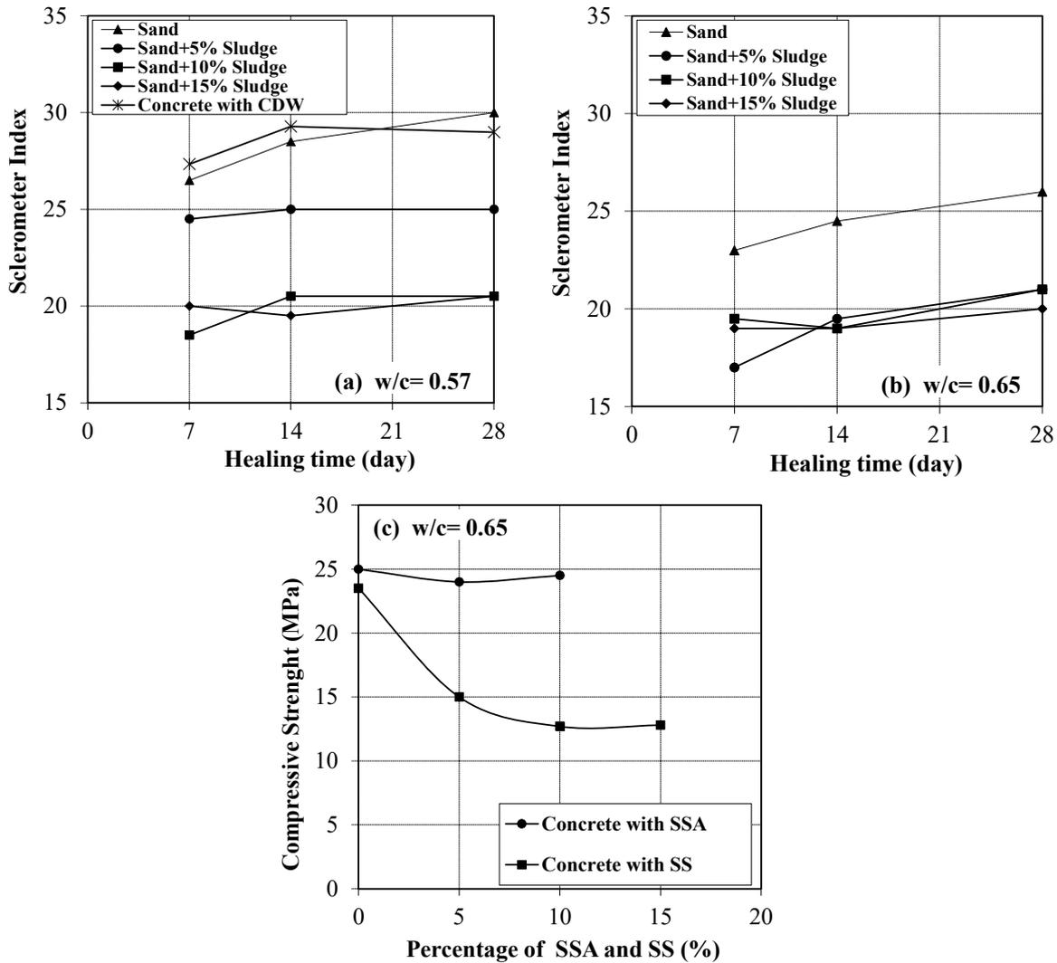
**Figure 8.** Compressive strength versus healing time: (a) conventional concrete, with sewage sludge and with CDW [27], w/c = 0.57; (b) conventional concrete with sewage sludge, w/c = 0.65.; and (c) concrete with sewage sludge (SS) and sewage sludge ash (SSA) [23], w/c = 0.65.
