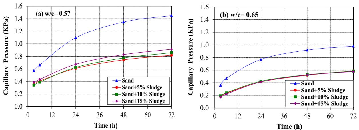
**Figure 9.** Capillary water absorption pressure versus time, with conventional concrete and concrete with sewage sludge: (a) for the ratio w/c = 0.57; and (b) for the ratio w/c = 0.65.
