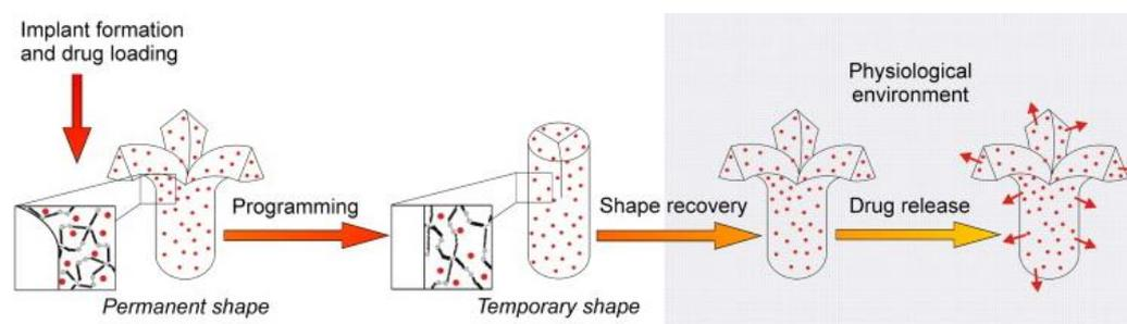
**Figure 5.** Programming of shape-recovery of polyester urethane shape memory polymer network in physiologic medium and temperature, and controlled drug release. Reprinted with permission from [84].
