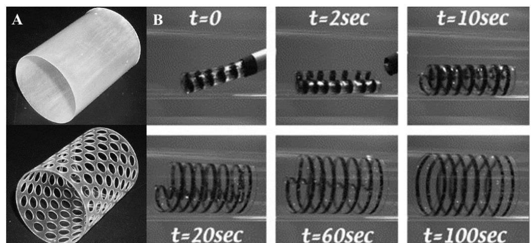
**Figure 4.** Photo sequence of shape memory polymer stent and its recovery. Solid and 50% perforated stents (A). The stent packaged in an 18 Fr. Catheter expands to 22 mm in a 37 °C water bath (B). Reprinted with permission from [73].
