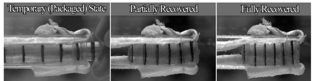
**Figure 6.** A shape memory polymer cylindrical that expands at body temperature. Reprinted with permission [93].
