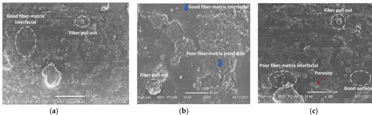
Figure 9. SEM image of unidirectional enset/sisal hybrid composite (a) untreated; (b) 5% NaOH-treated; and (c) 10% NaOH-treated.
