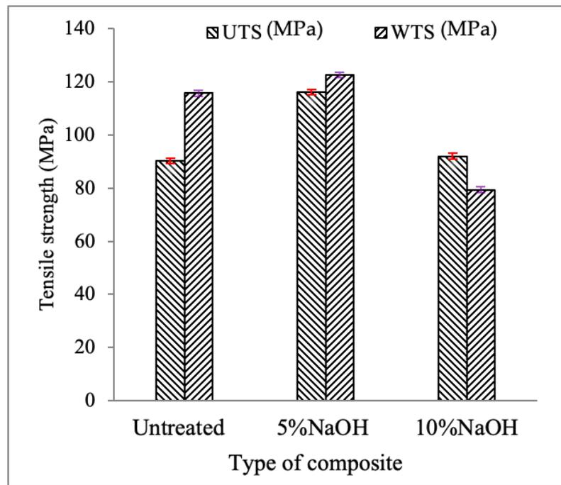
Figure 4. Tensile strength plot of unidirectional (UTS) and woven (WTS) composites.
