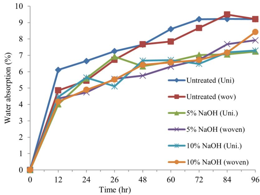
Figure 7. Water absorption test result.
