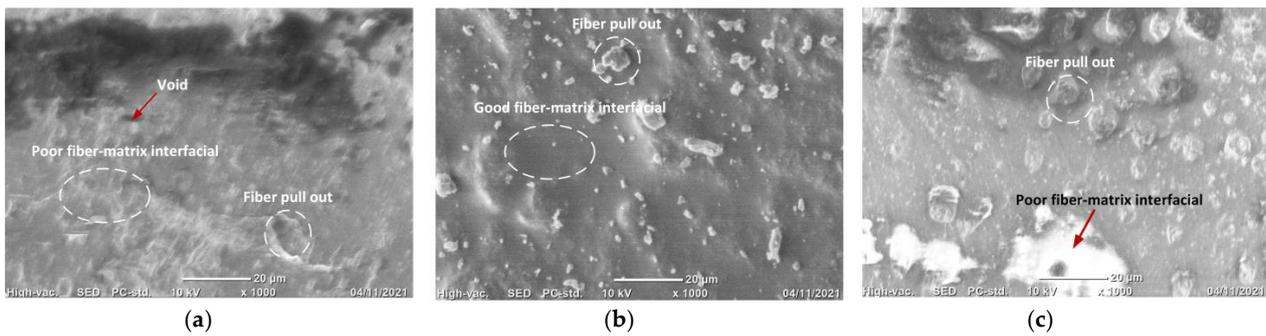
Figure 8. SEM image of woven enset/sisal hybrid composite (a) untreated; (b) 5% NaOH-treated; and (c) 10% NaOH-treated.
