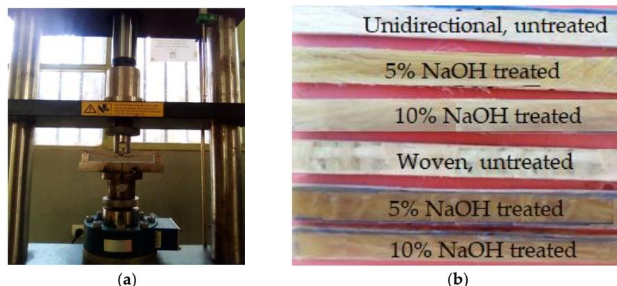
**Figure 3.** (a) Bending test setup in the UTS machine and (b) flexural test specimens.
