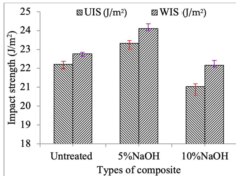
**Figure 6.** The impact strength of unidirectional (UIS) and woven (WIS) composites.
