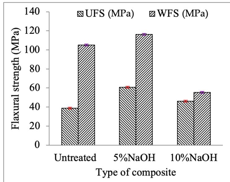
Figure 5. The flexural strength of unidirectional (UFS) and woven (WFS) composites.
