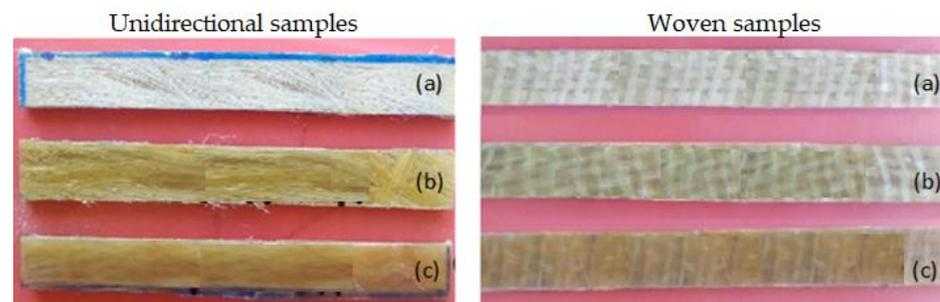
**Figure 2.** Unidirectional (L) and woven orientation (R) types of (a) untreated; (b) 5% NaOH-treated; and (c) 10% NaOH-treated E/S hybrid composites.
