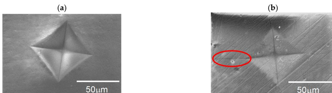
**Figure 18.** Vickers hardness indentation impression on  $ZrO_2$ -rich surfaces of the FGMs with PCA (20%) before (a) and after (b) cyclic thermal shock tests.
