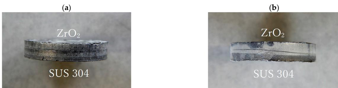
Figure 16. 3-layered (a) and 2-layered (b) samples just after SPS.
