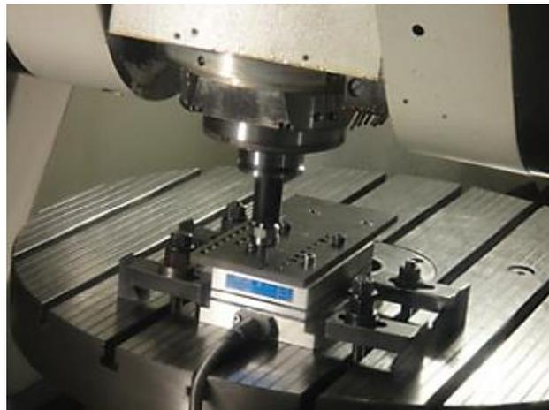
**Figure 12.** Experimental setup for measuring the cutting forces in helical milling [121]. Reproduced with permission from Springer.
