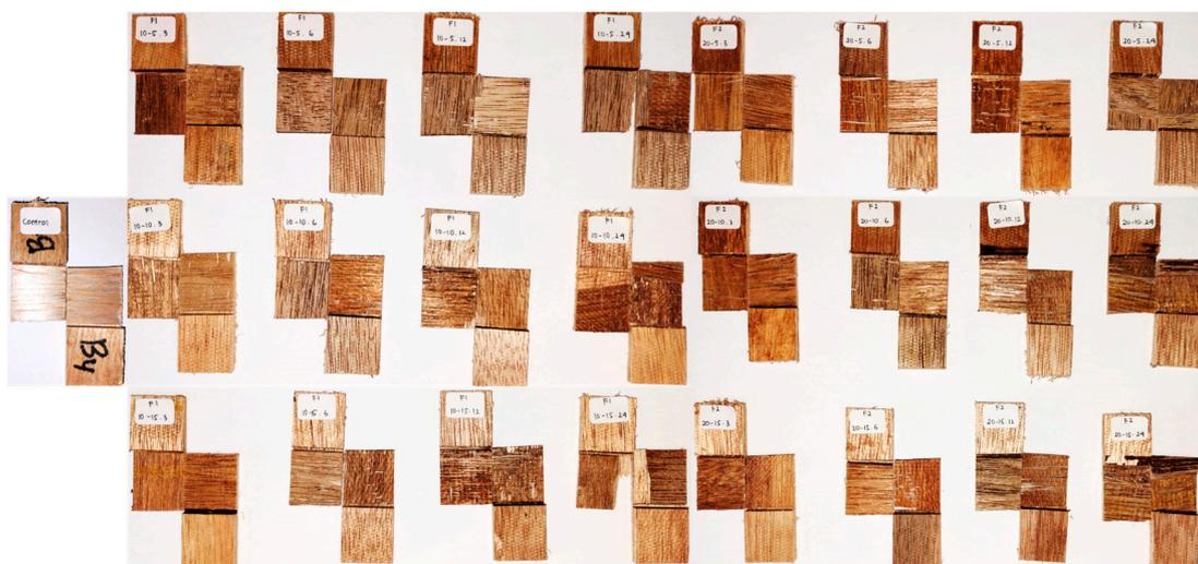
**Figure 8.** The wood failure images of plywood bonded with PVOH–tannin–hexamine-based adhesives.
