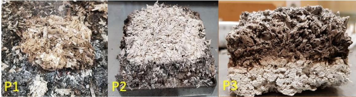
Figure 3. Samples after exposure to heat in the cone calorimeter test.
