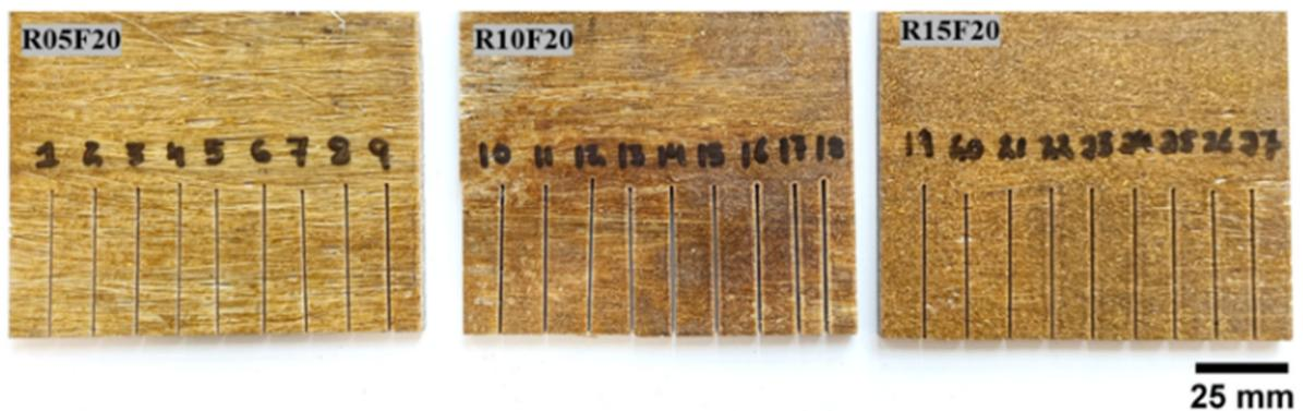
**Figure 3.** AWJ-machined hybrid RS<sub>p</sub>/FF test samples.
