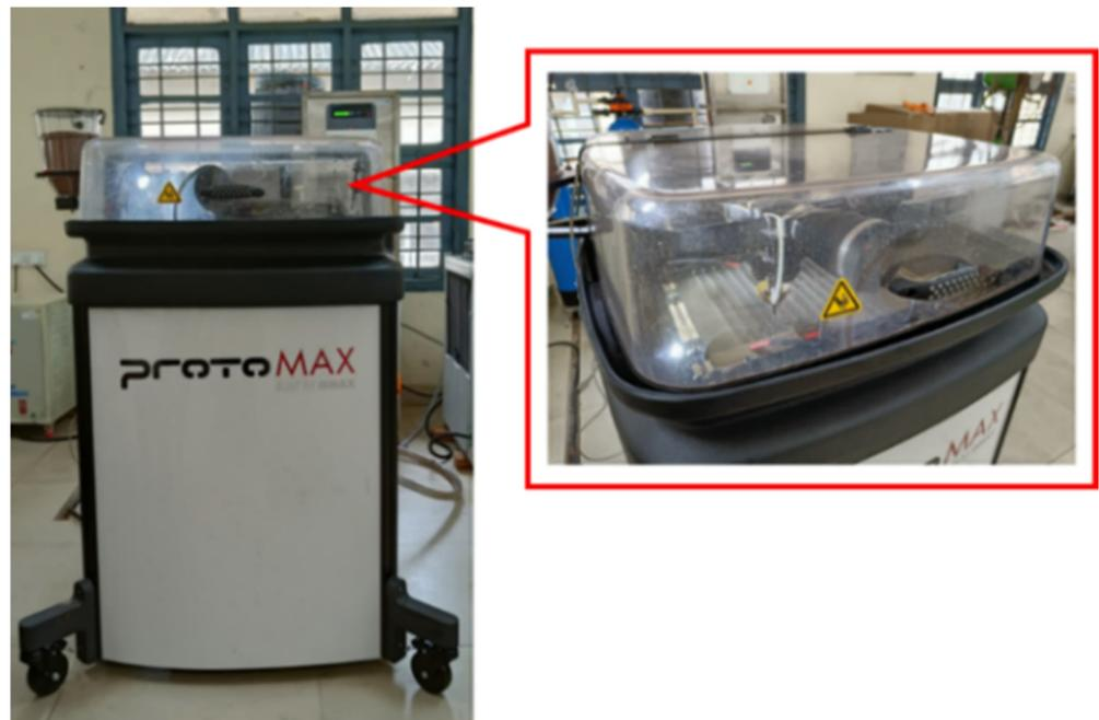
**Figure 2.** Abrasive water jet machine.
