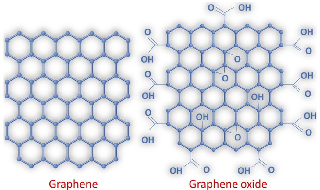
**Figure 1.** Graphene and graphene oxide.
