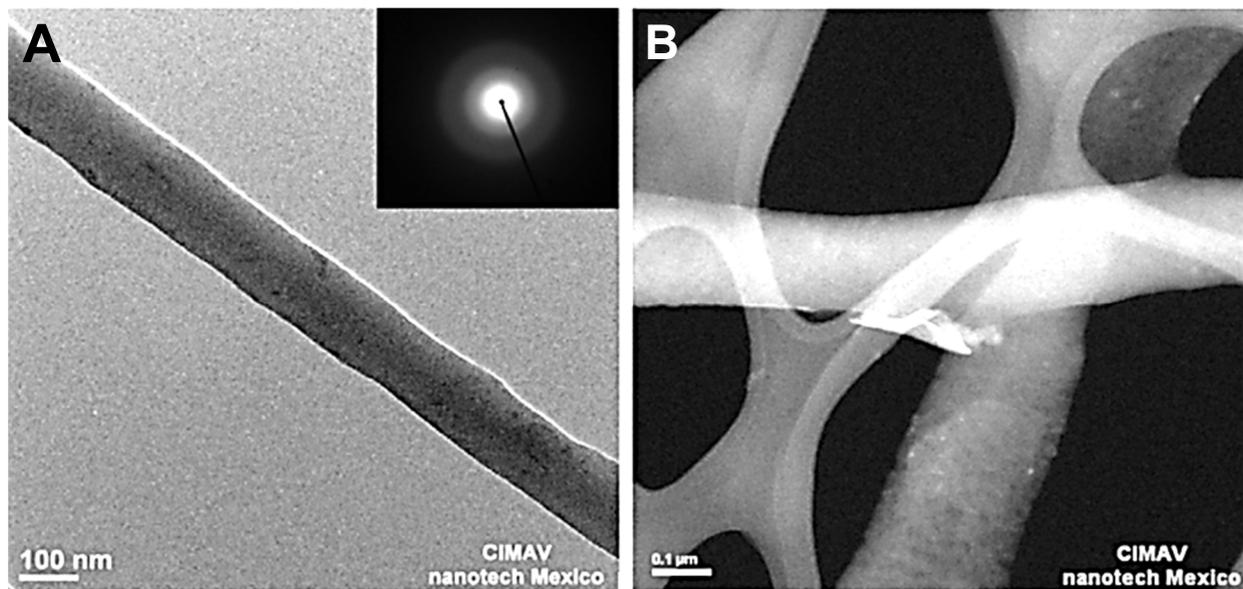
**Figure 8.** (A) TEM bright field image of nylon 6 nanofiber; (B) STEM Z-contrast image showing two nanocomposite nanofibers containing GOFT layers [150]. STEM = scanning transmission electron microscopy; GOFT = nitroxide-functionalized graphene oxide layers. Reproduced with permission from Elsevier.
