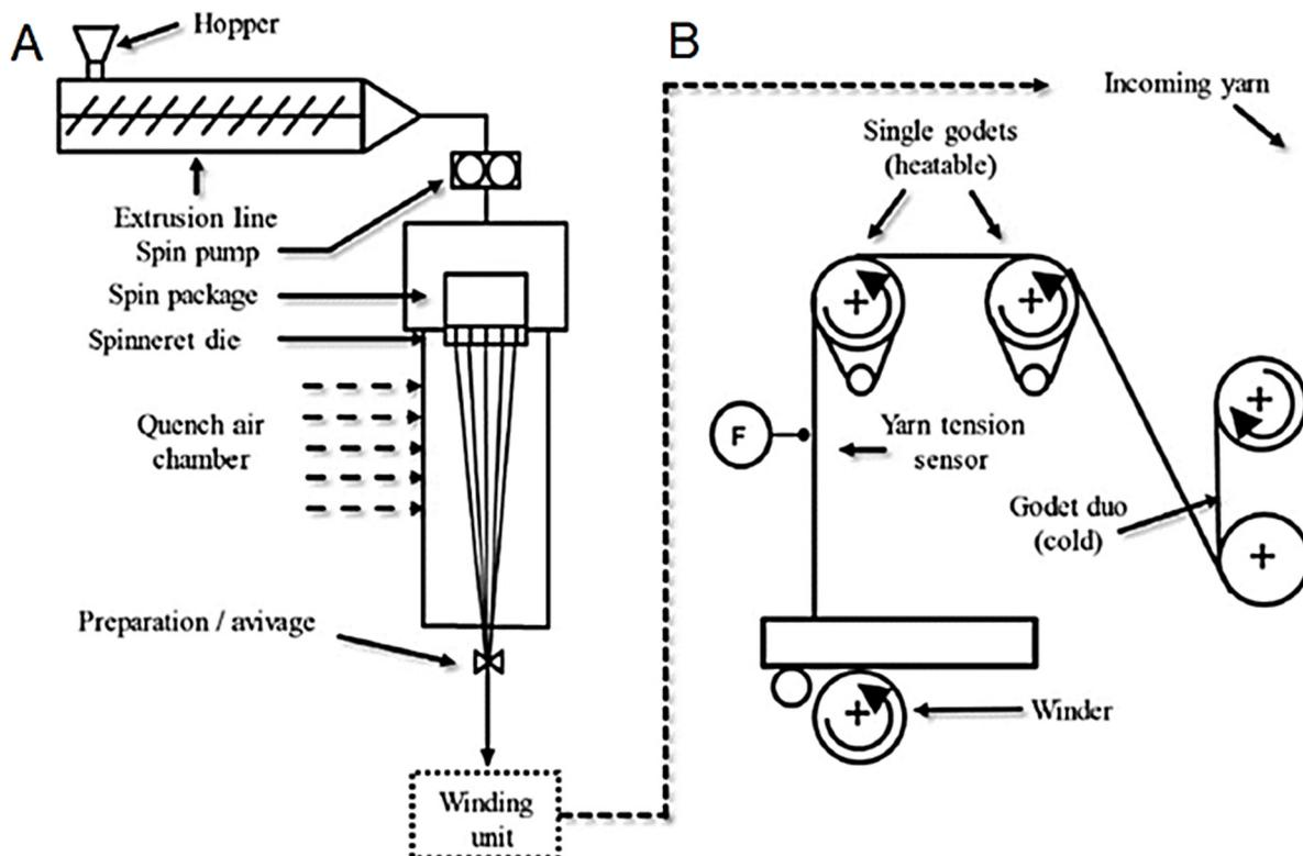
**Figure 9.** (A) The pilot-scale extrusion line and (B) winding system used to produce graphene-modified polyamide 6 yarns [151]. Reproduced with permission from Elsevier.
