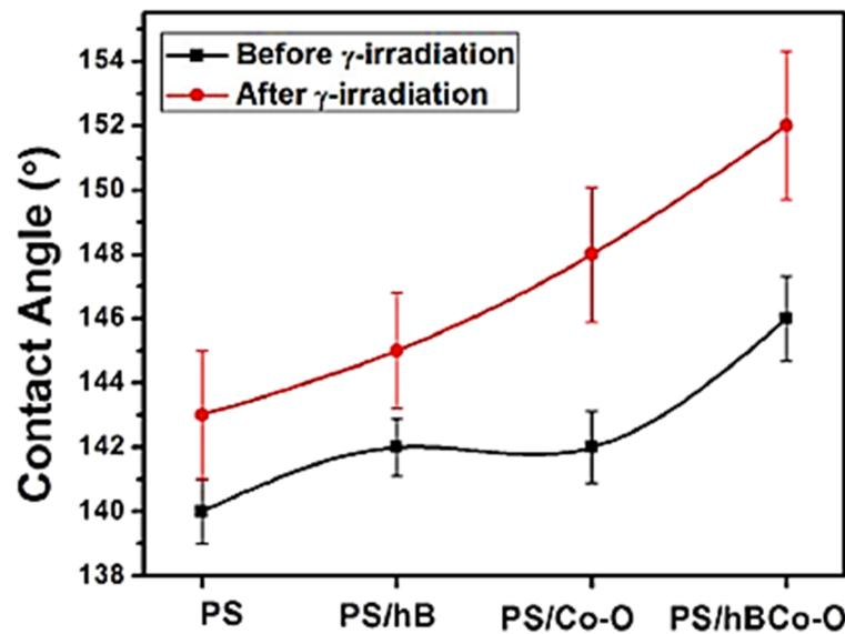
**Figure 10.** Contact angle of nanocomposite nanofibers before and after gamma irradiation [158]. PS = polystyrene; PS/Co-O = PS/Co<sub>3</sub>O<sub>4</sub> at 1 wt.%; PS/hB = polystyrene/hexagonal boron nitride at 1 wt.%; PS/hBCo = PS/hexagonal boron nitride/Co<sub>3</sub>O<sub>4</sub> at 1 wt.%. Reproduced with permission from MDPI.
