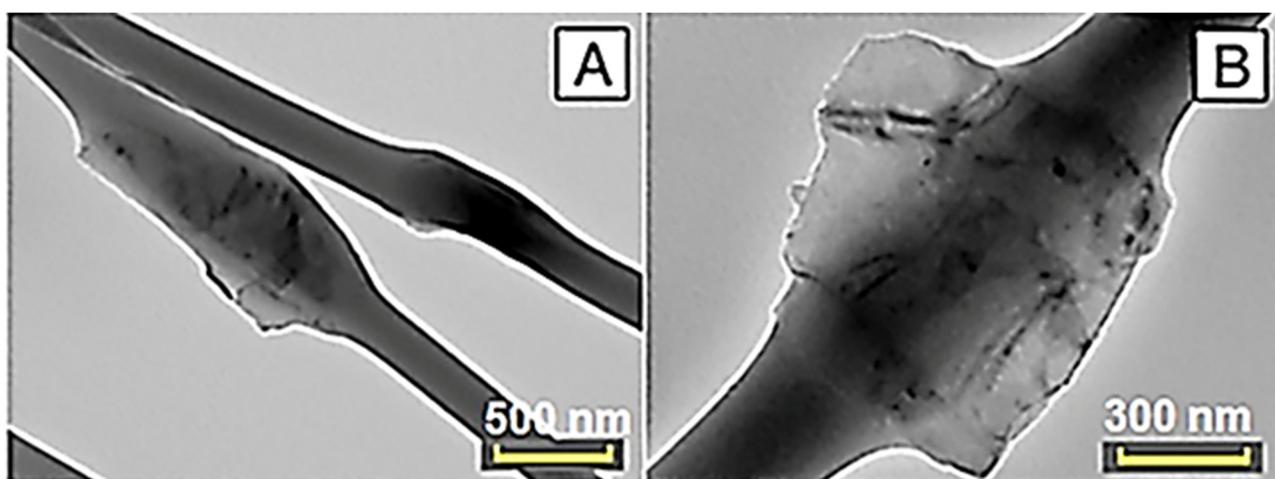
**Figure 6.** TEM micrographs of nanofibrous mats with (A) 5 wt.% graphene and (B) 15 wt.% graphene [148]. Reproduced with permission from Elsevier.
