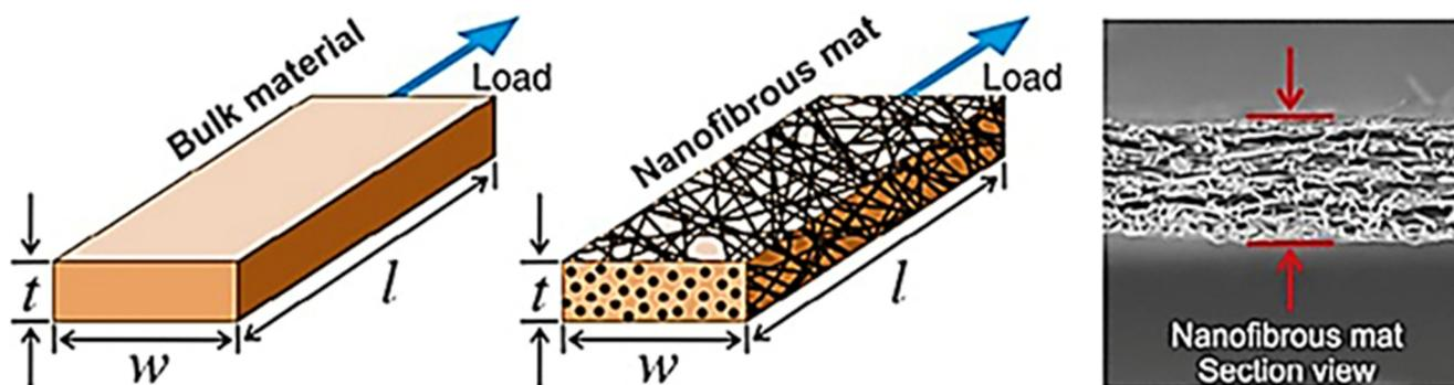
**Figure 7.** Schematic representation of bulk versus nanofibrous material and cross-sectional area of nanofibrous material [148]. Reproduced with permission from Elsevier.
