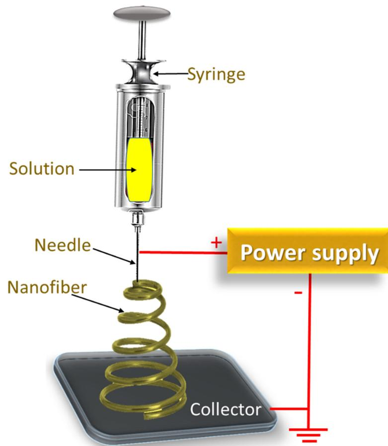
**Figure 2.** Electrospinning setup.
