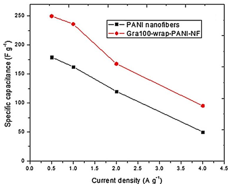
**Figure 5.** Specific capacitance of polyaniline (PANI) and graphene-wrapped polyaniline nanofibers (Gra100-wrap-PANI-NF) vs. varying current densities [134]. Reproduced with permission from Elsevier.
