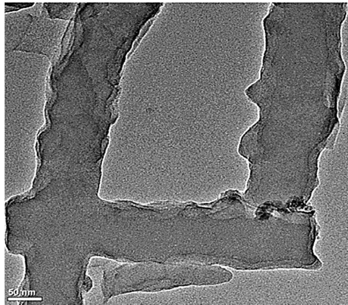
**Figure 4.** Transmission electron microscopy (TEM) image of graphene-wrapped polyaniline nanofibers [134]. Reproduced with permission from Elsevier.
