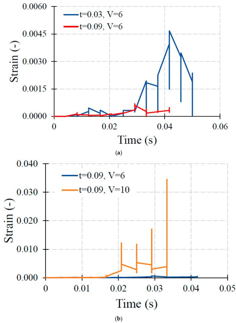
**Figure 12.** Effect of crucial parameters on the behaviour of ships containing SCS composite plates: (a) effect of layers' thickness for V6; (b) effect of drop velocity of the ship.
