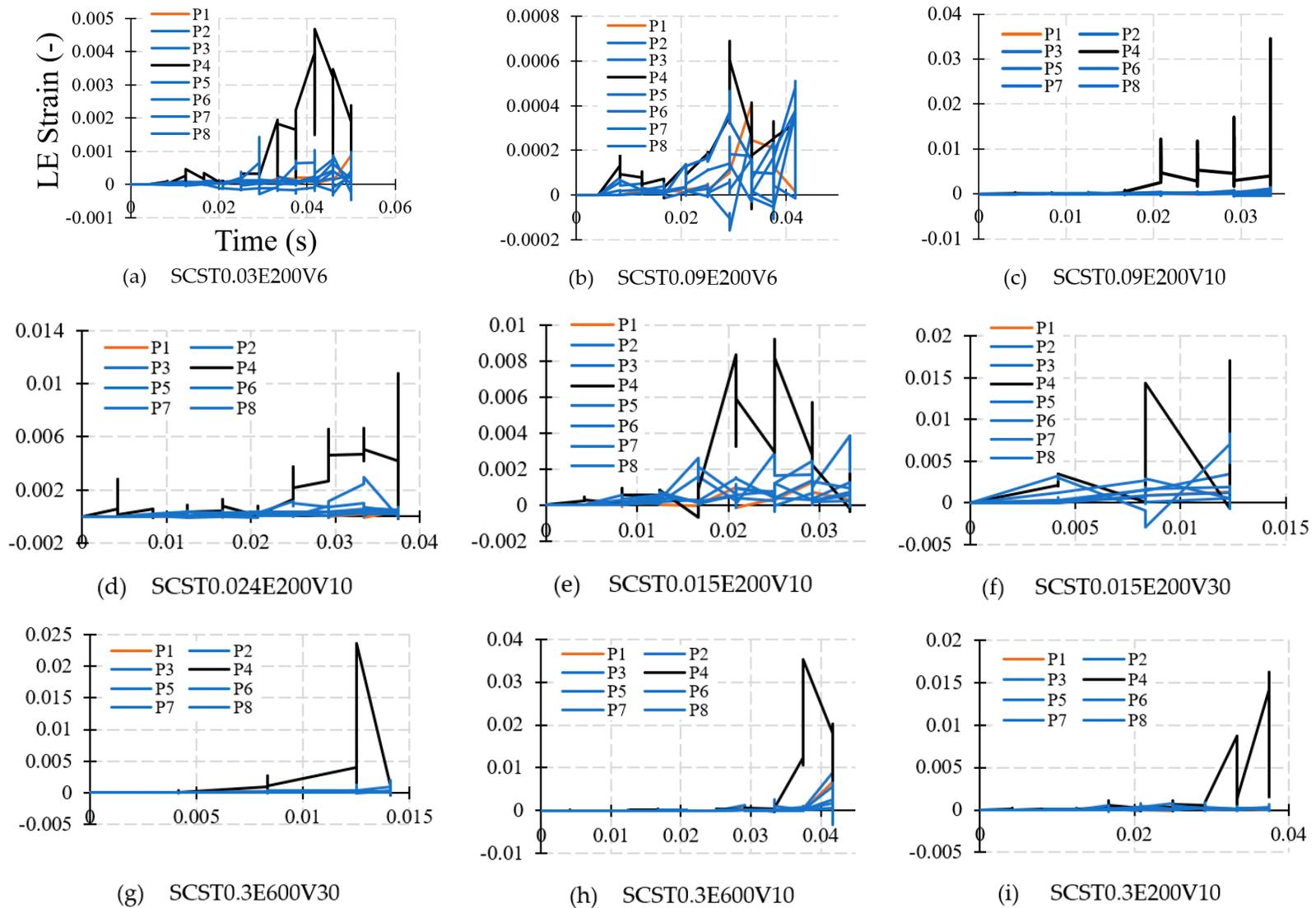
**Figure 8.** Strain of points located at the external layer of ship model (axis titles of graphs are the same as (a) SCST0.03E200V6; (b) SCST0.09E200V6; (c) SCST0.09E200V10; (d) SCST0.024E200V10; (e) SCST0.015E200V10; (f) SCST0.015E200V30; (g) SCST0.3E600V30; (h) SCST0.3E600V10; (i) SCST0.3E200V10.
