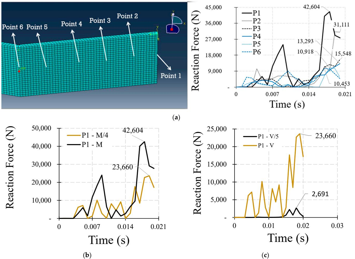
**Figure 3.** Parametric study of the wedge-shaped structure: (a) finding critical point; (b) effect of the weight of the structure; (c) effect of impact velocity.
