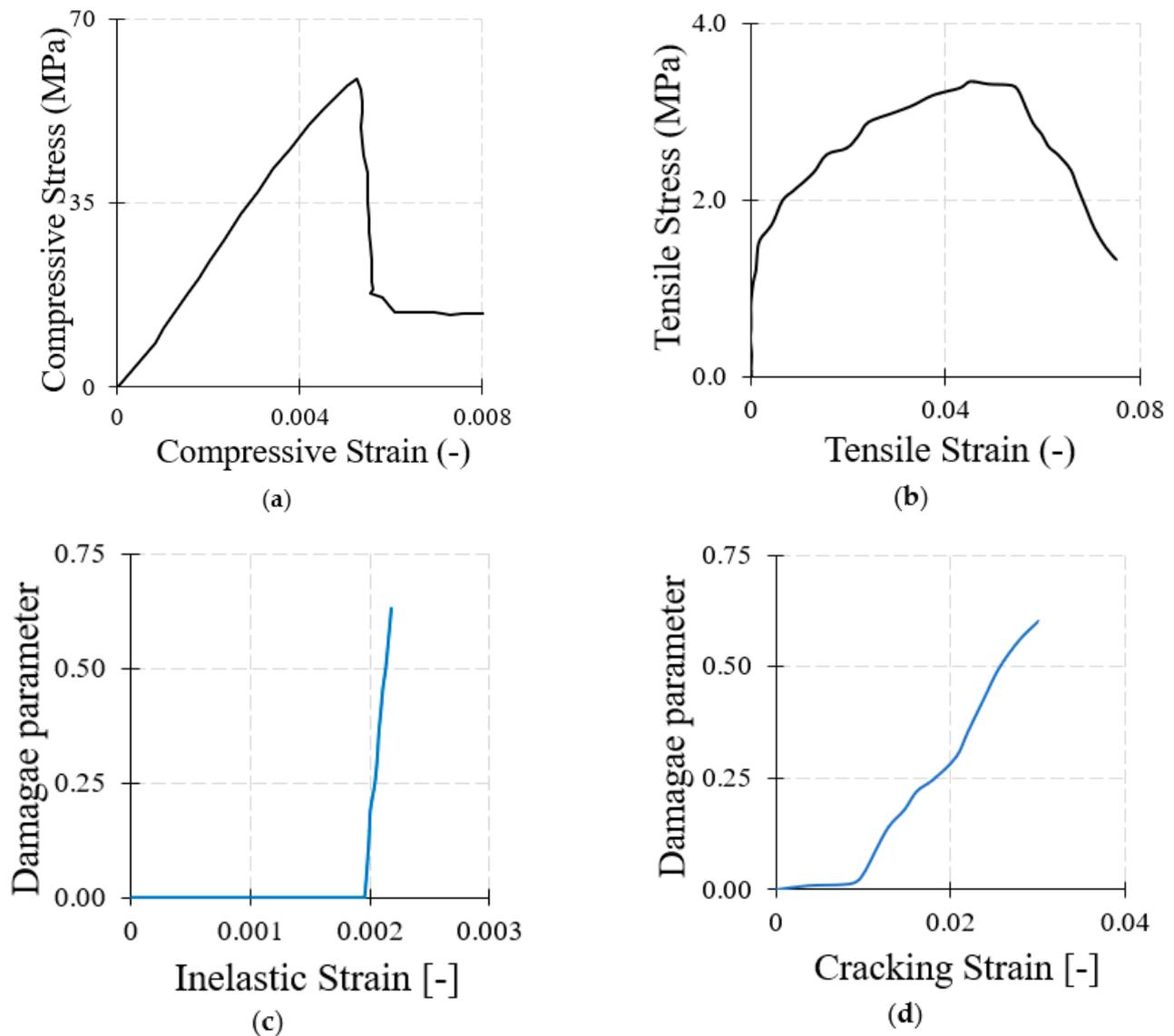
**Figure 7.** CDP stress–strain curves and damage parameters for ultra-lightweight high-ductility cementitious composite used in the present study: (a) compression stress–strain curve extracted from Liu et al. (2016) [27]; (b) tension stress–strain curve extracted from Huang et al. (2021) [28]; (c) compressive damage parameters; (d) tensile damage parameters.
