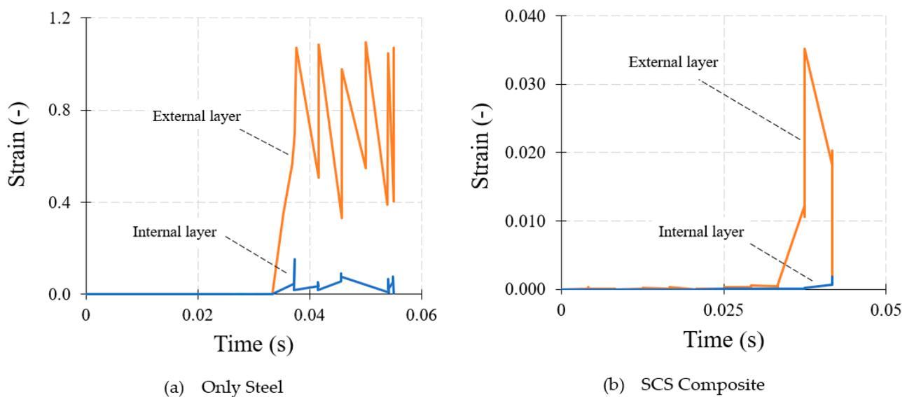
**Figure 10.** The strain of the bottom structure of the ship: (a) SCS composites with E600V10; (b) only steel plate with E600V10.
