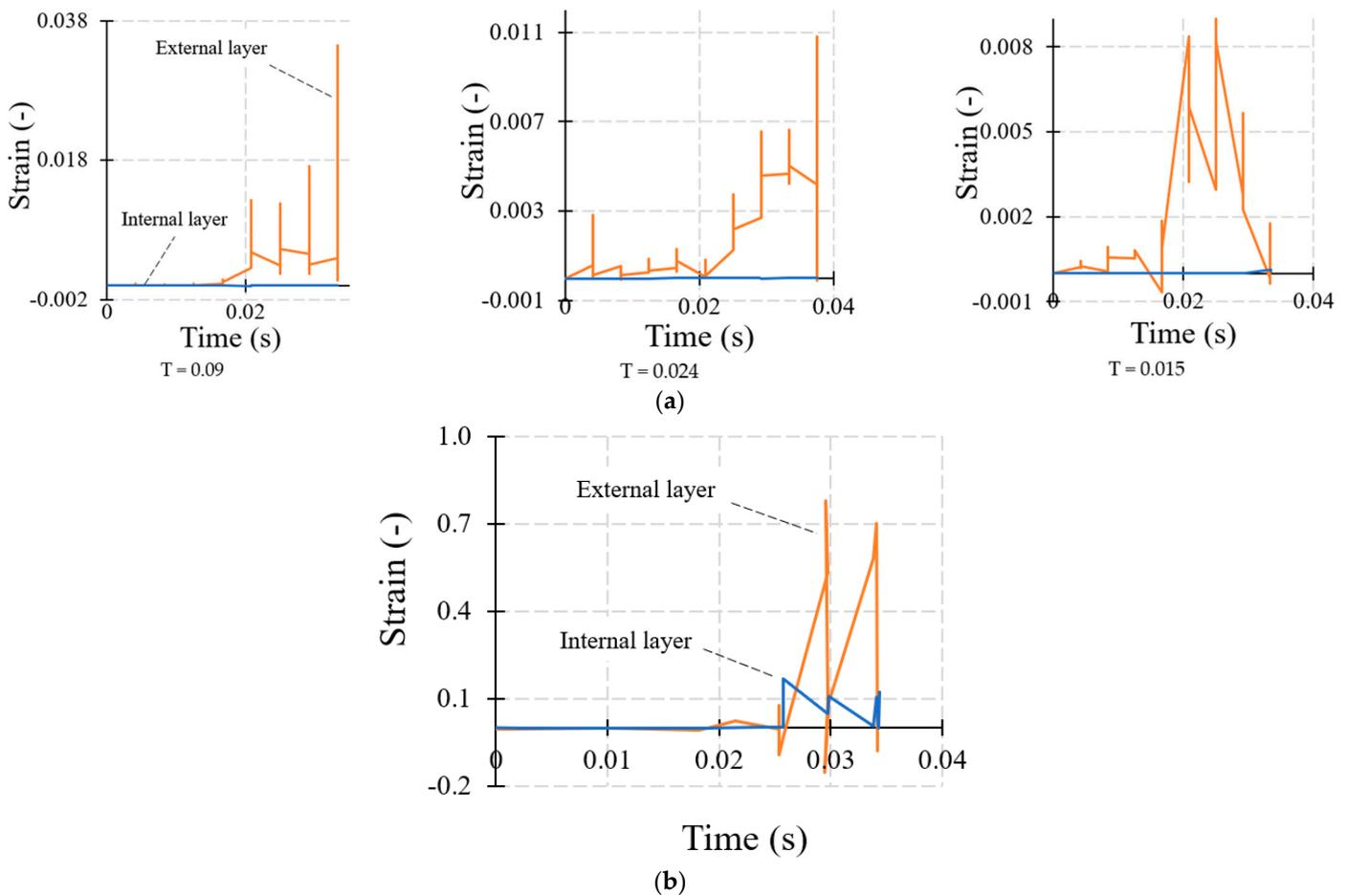
**Figure 9.** Strain of the bottom structure of the ship: (a) SCS composites with E200V10; (b) only steel plate with E200V10.
