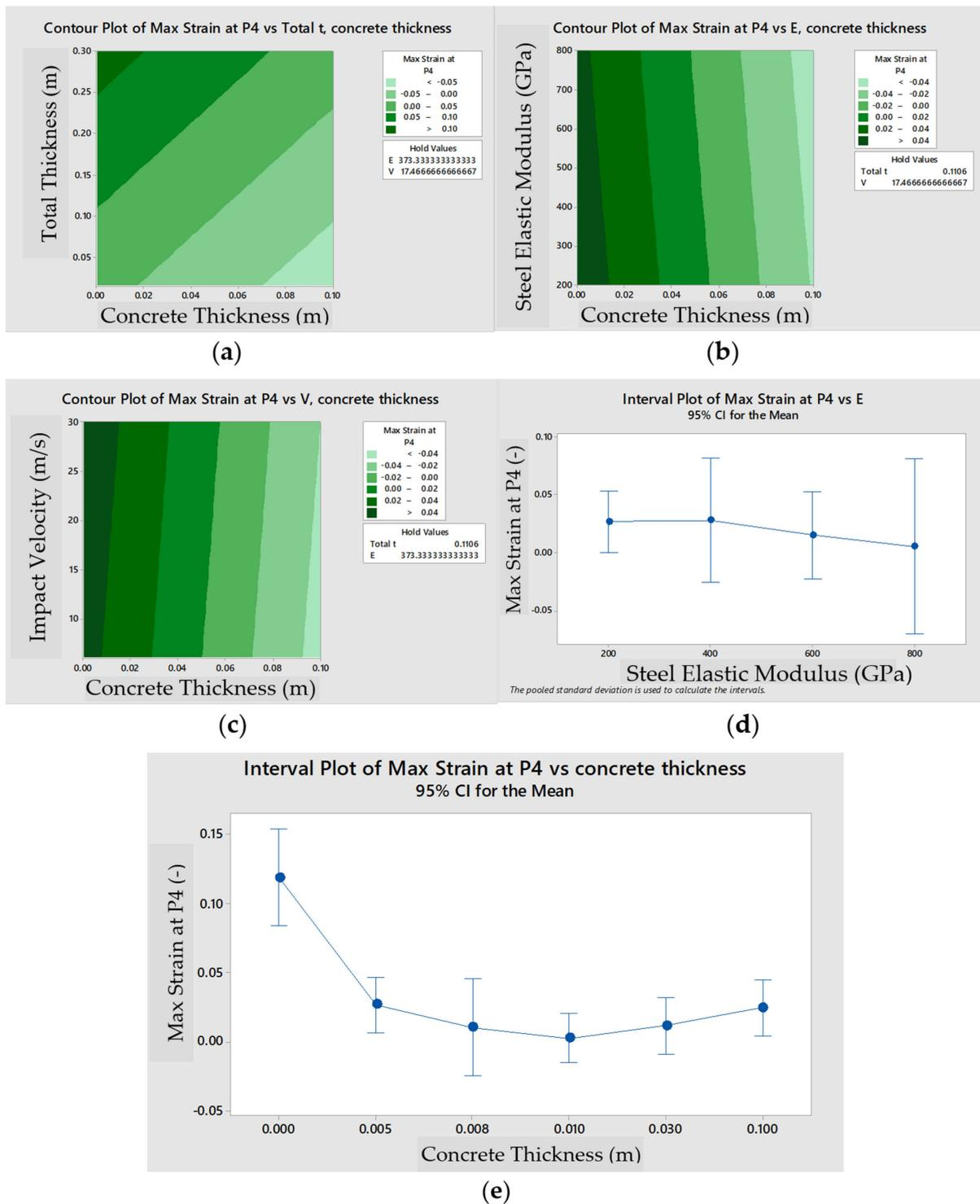
**Figure 14.** ANOVA analysis to determine the importance of parameters in ships containing SCS composite plate: (a) effects of total thickness and concrete thickness on the maximum strain; (b) effects of steel elastic modulus and concrete thickness on the maximum strain; (c) effects of impact velocity and concrete thickness on the maximum strain; (d) one-way effect of steel elastic modulus on the maximum strain; (e) one-way effect of concrete thickness on the maximum strain.
