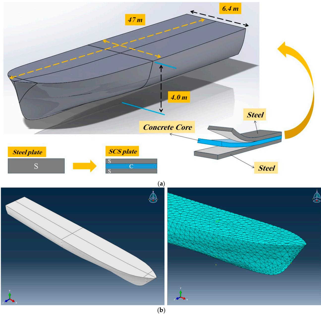
**Figure 4.** Layout of the present study regarding numerical modelling ship: (a) solid model of the ship; (b) Abaqus model.
