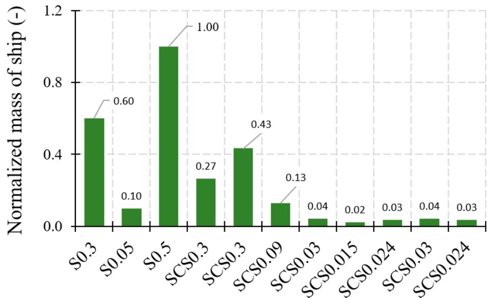
**Figure 13.** Mass of SCS plates compared to only steel plates (normalised with S0.5).
