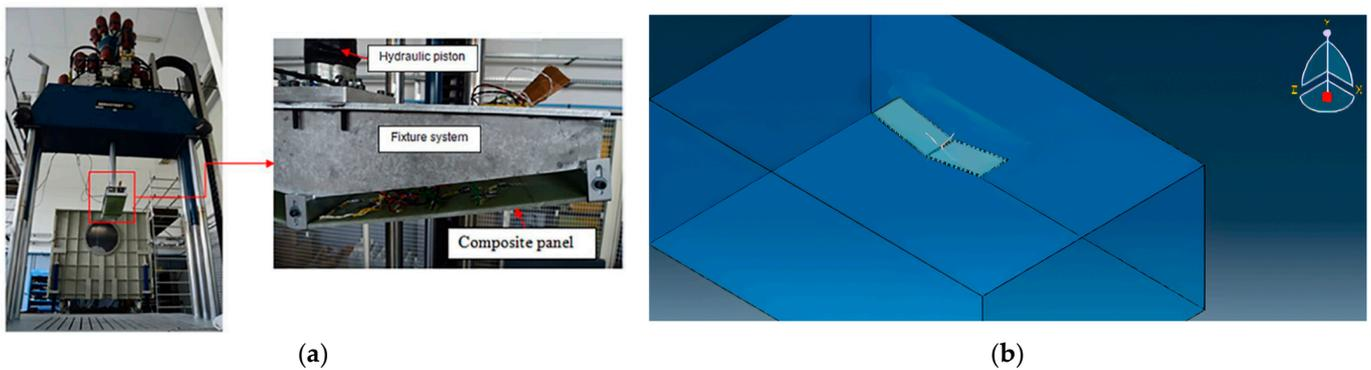
Figure 1. Validation of the numerical study: (a) experimental specimen tested by Hassoon et al. (2018) [25]; (b) numerical model in the present study.
