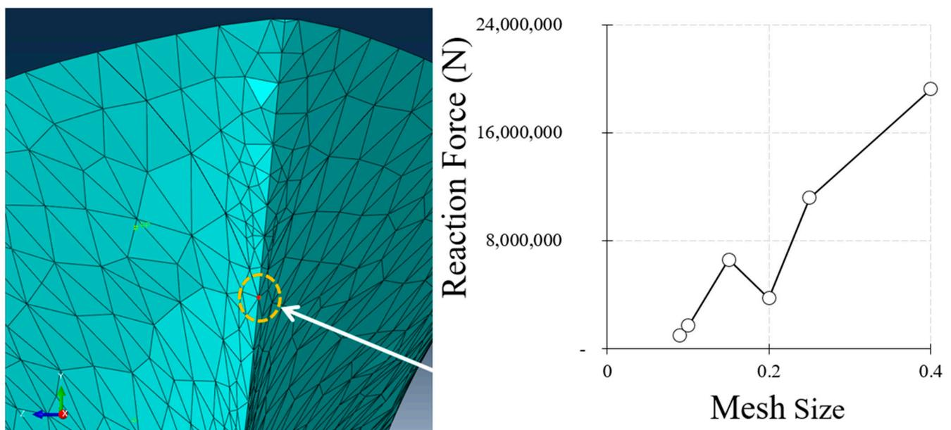
**Figure 5.** Mesh sensitivity analysis for Abaqus model of ship.
