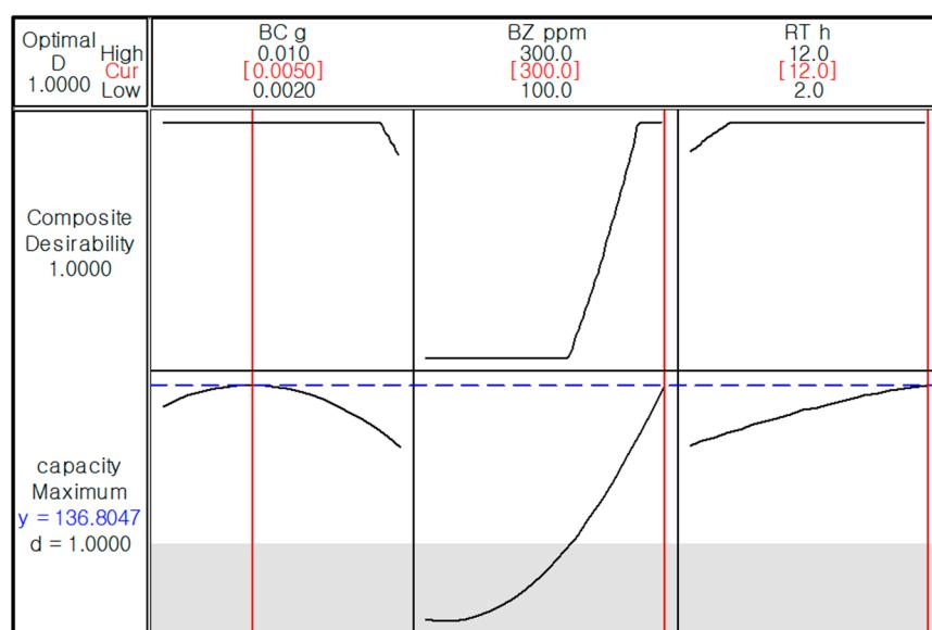
**Figure 6.** Predicted values of different variables (KB-BC550 dose (g), reaction time (RT, h), and benzene concentration (ppm)) for optimum adsorption capacity. Blue line is the chosen conditions for the optimum adsorption capacity of benzene. Red line is the optimal conditions of variables.
