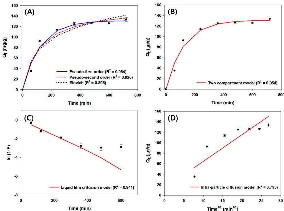
**Figure 3.** Kinetic studies of KB-BC550 for benzene adsorption by fitting pseudo-first-order, pseudo-second-order, and Elovich model (A), two-compartment model (B), liquid film diffusion model (C), and intra-particle diffusion model (D). [Conditions] For benzene, 4.5 mL of 300 ppm; 0.005 g BC; initial pH of 7; 1–12 h (60, 120, 240, 360, 480, 600, 720 min). The experiments were conducted in triplicate.
