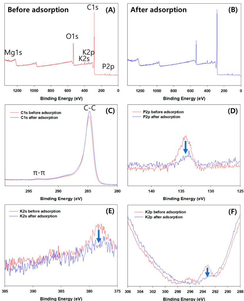
**Figure 4.** XPS survey scan (A,B), C1s (C), P2p (D), K2s (E), and K2p (F) of KB-BC550 before and after benzene adsorption. Arrow means the decrease of peak.
