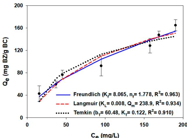
**Figure 2.** Isotherm studies of KB-BC550 for benzene adsorption by Langmuir, Freundlich, and Temkin isotherm models. [Conditions] For benzene, 4.5 mL of 300 ppm; 0.003–0.03 g BC (0.003, 0.004, 0.005, 0.01, 0.015, 0.02, 0.03 g); initial pH of 7; 24 h. The experiments were conducted in triplicate.
