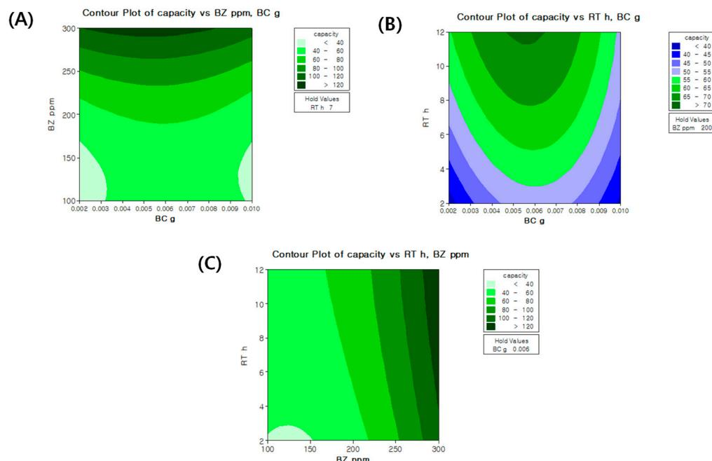
**Figure 5.** Two-dimensional contour plots showing effects of KB-BC550 dose (g), reaction time (RT, h), and benzene concentration (ppm) on adsorption capacity of benzene (BZ) (A–C).
