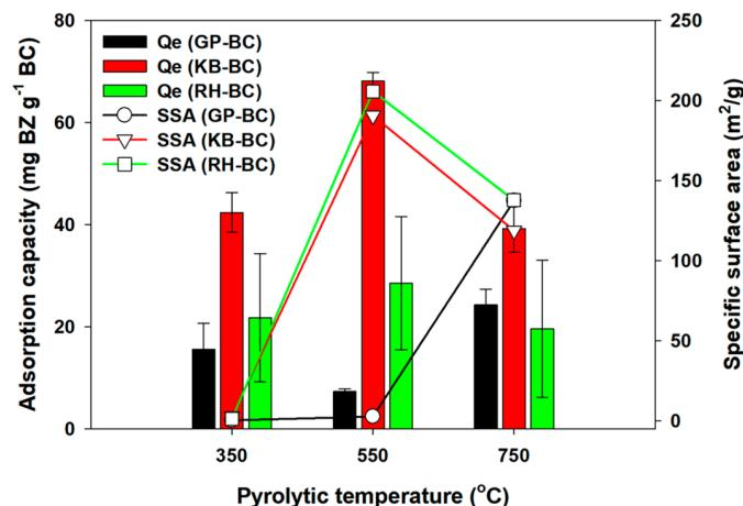
**Figure 1.** Comparison of adsorption capacity ( $Q_e$ ) and specific surface area (SSA) of different biochars (GP-BCs, KB-BCs, and RH-BCs) produced at different pyrolytic temperatures (350 °C, 550 °C, and 750 °C). [Conditions] For benzene, 4.5 mL of 200 ppm; 0.005 g BC; initial pH of 7; 48 h. The experiments were conducted in triplicate.
