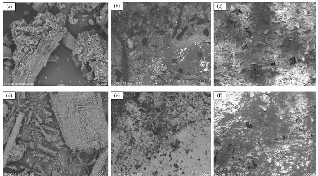
**Figure 2.** SEM images of (a) pure cow pie powder at 100 μm magnification; (b) OM37 blend PCM at a 20/50 ratio at 200 μm magnification; (c) OM42 blend at a 20/50 ratio at 200 μm magnification; (d) pure cow pie powder at 500 μm magnification; (e) OM37 blend at 20/50 ratio at 500 μm magnification; (f) OM42 blend at 20/50 ratio at 500 μm magnification.
