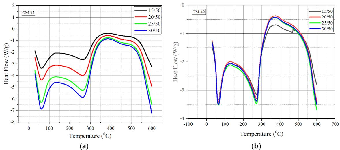
**Figure 4.** DSC curves of (a) OM37 blend and (b) OM42 blend.
