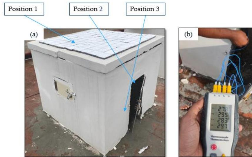
**Figure 6.** (a) Physical setup built for testing the tiles; (b) temperature measurement using a thermocouple.
