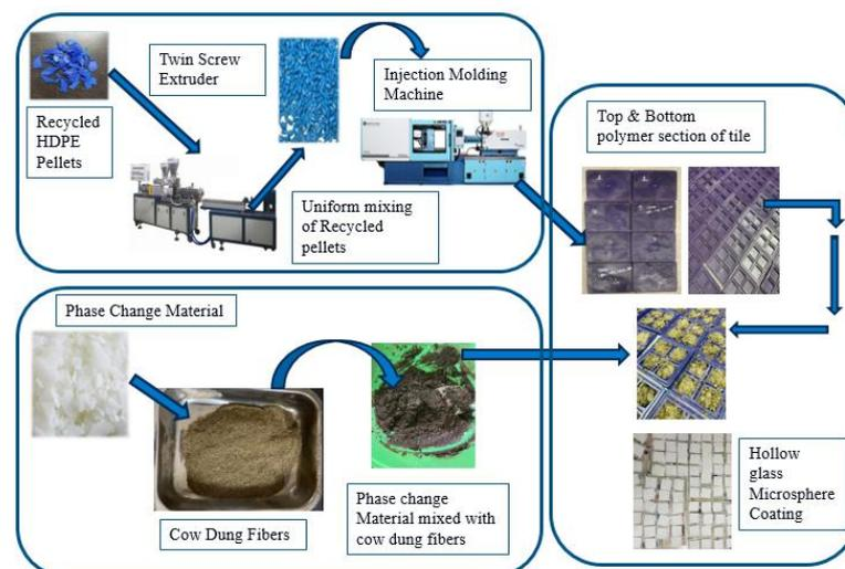
**Figure 1.** Schematic flowchart of the preparation of novel recycled plastic roof tiles.
