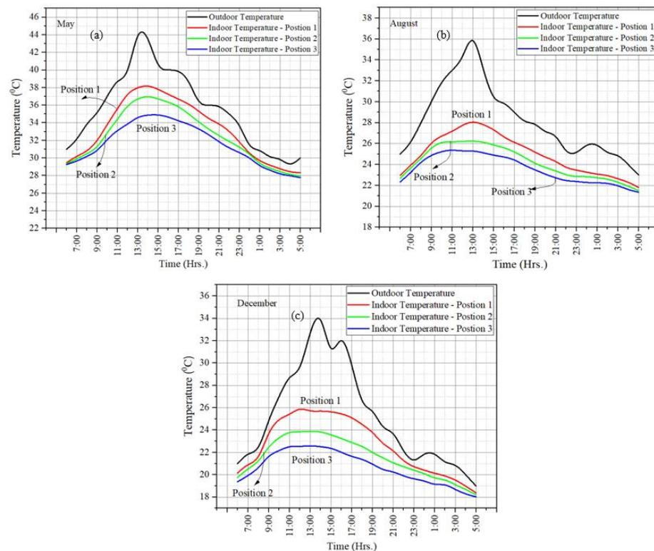
**Figure 7.** Real-time temperature distribution of recycled plastic roof tiles in (a) summer (May), (b) rainy (August), and (c) winter (December) seasons.
