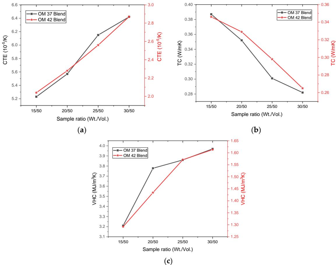
Figure 5. (a) Coefficient of thermal expansion, (b) thermal conductivity, (c) volumetric heat capacity.
